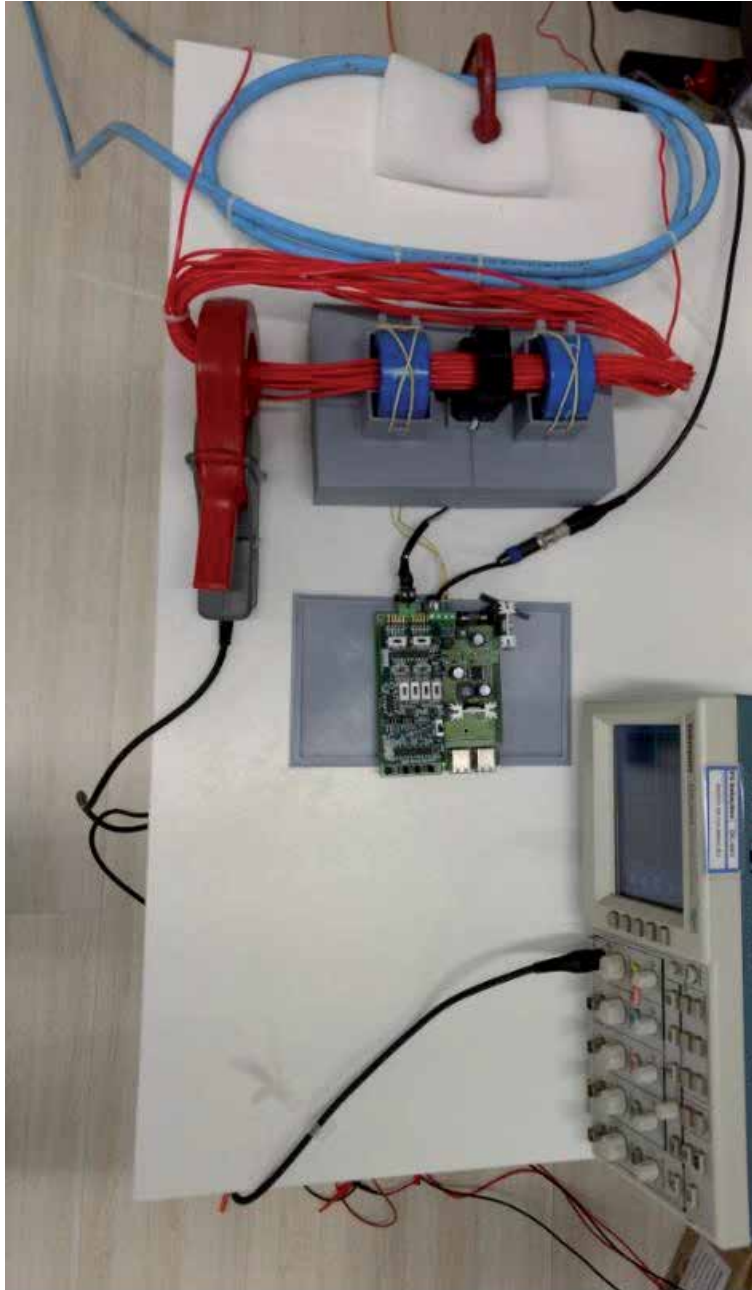
Figure 17. Assembly of the starter test for motor without soft starter.
