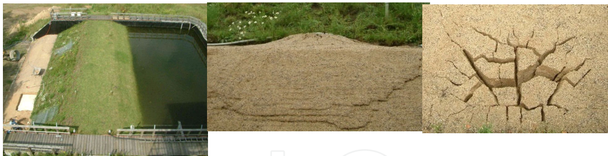
Figure 4. Laboratory dike at the University Hannover, Germany and soil displacement in the dike.
