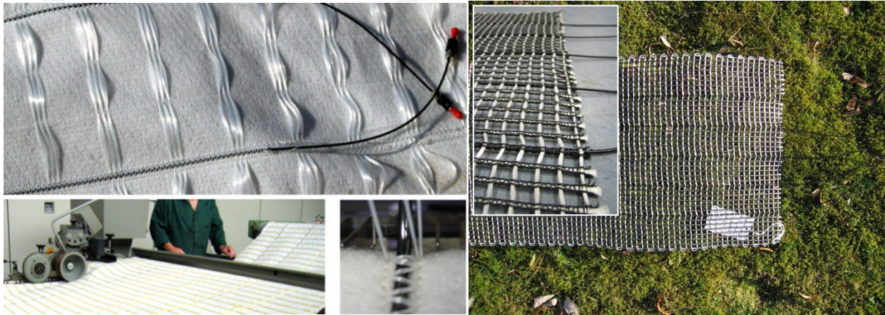
Figure 11. Integration of POF into nonwoven geotextiles at STFI e.V. (left) and a geogrid containing POF (right).
