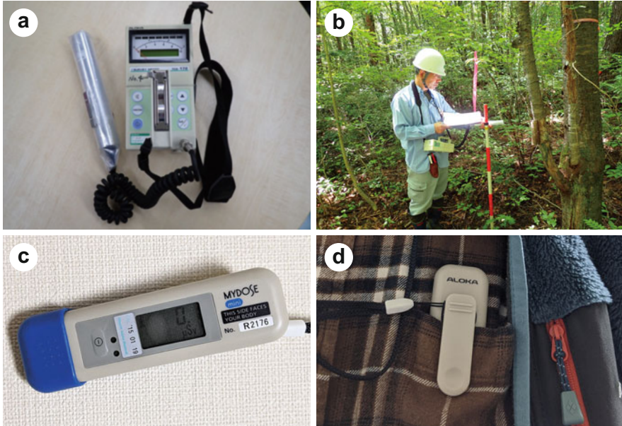
Fig. 2.5 Various dosimeters and examples of their use. (a) a survey meter (air dose rate meter), (b) measurement of air dose rates in forests, using a pole with scale to measure at a fixed height, (c) personal dosimeters, and (d) personal dosimeters worn with the clip side facing outward from the body (Courtesy of Wataru Sakashita, the Forestry and Forest Products Research Institute (a, b) , and photos taken by the author (c, d) )
