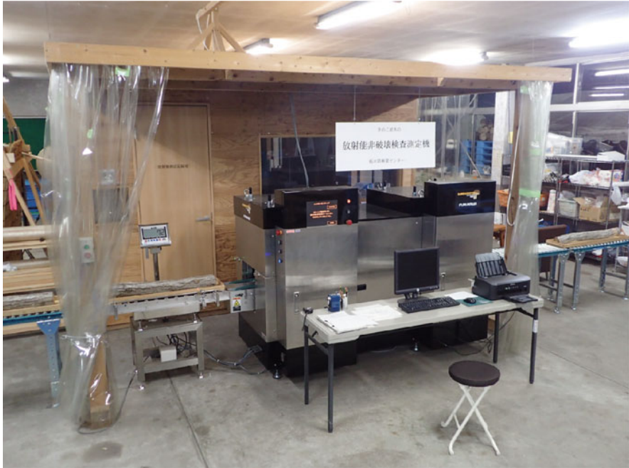
Fig. 6.31 A non-destructive inspection machine for logs (Courtesy of Yoshinori Imai, Tochigi Forestry Center)
