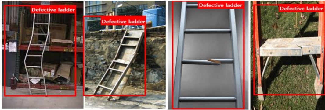
Figure 5: Example of Ladder for Monitoring with Intervals
