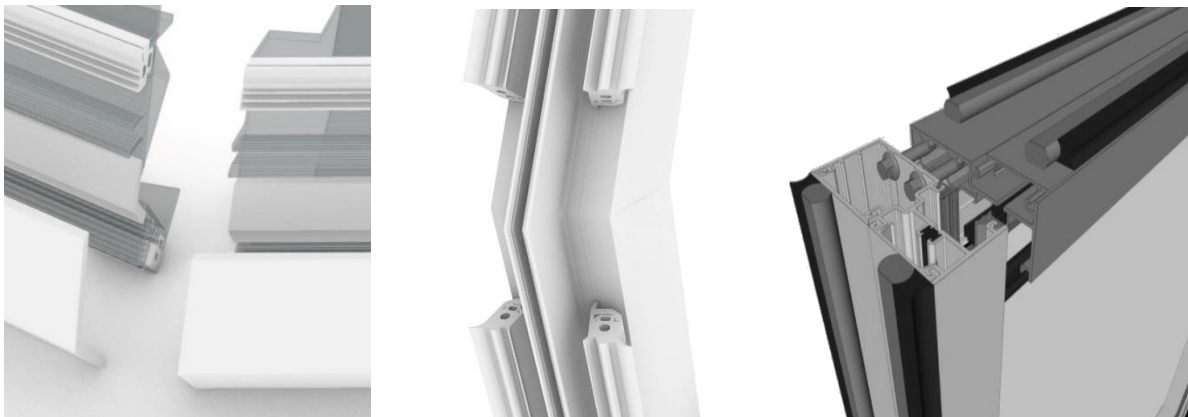
Figure 3: Components of a façade node (left, center), Window in LOD 400 (right) source: BIMForum
