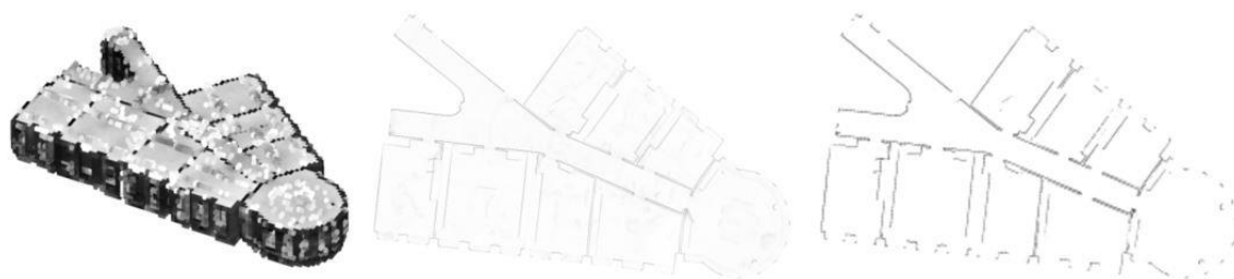
Figure 2: Steps for wall extraction. From left to right: The input point cloud is voxelized and occupied voxels marked. The sum of occupied voxels in vertical direction forms a 2D density map. Thresholding the density map reveals the location of walls.
