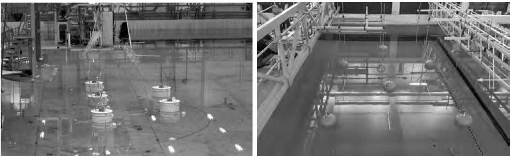
Figure 9.4: Pictures of two experimental campaigns that have been carried out on wave farms in wave tank laboratories. (a) Wave farm consisting of five floating OWCs. Experiments carried out at the NTNU Trondheim basin [423]. (b) Wave farm consisting of six point-absorber buoys connected to linear damping PTOs. Carried out at the COAST laboratory OCEAN basin, Plymouth, UK [281].
