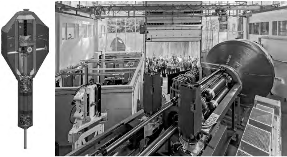
Figure 3.10: Point absorber applying a direct mechanical drive PTO, (image courtesy of CorPower Ocean.)
