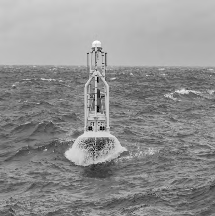
Figure 1.14: PB3 PowerBuoy ® WEC, developed by Ocean Power Technologies during commercial deployment in the North Sea, (image courtesy of Ocean Power Technologies).
