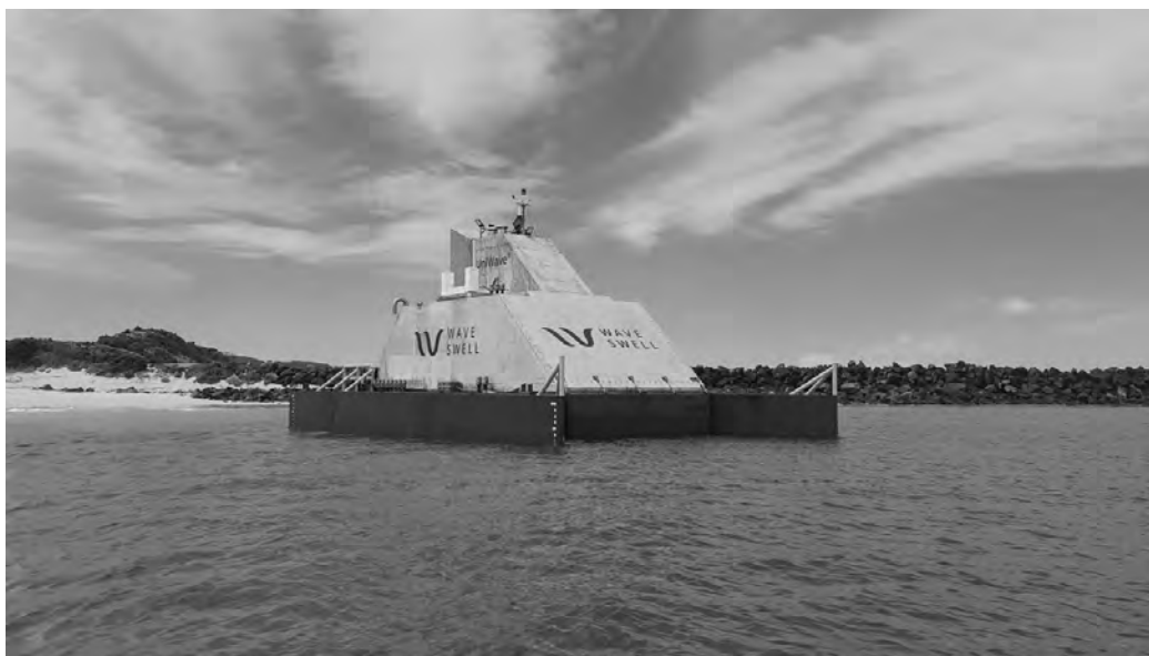
Figure 1.13: UniWave200, a 200 kW rated OWC developed by Wave Swell Energy, (image courtesy of Wave Swell Energy).
