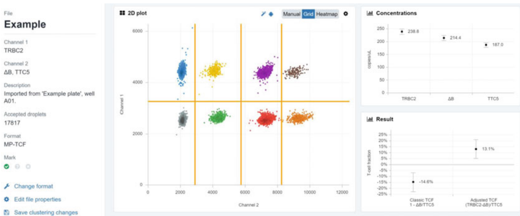
Fig. 6 Example of the analysis of our multiplex experimental setup in Roodcom WebAnalysis. Here, 20 ng DNA from a malignant melanoma is analyzed. In the panel “2D plot,” eight distinct clusters are detected that are used to calculate the concentrations of the individual targets (in the panel “Concentrations”). When the experimental format is set to “T cell multiplex” (MP-TCF), the T cell fractions according to the classic and adjusted model and their associated 95% confidence interval are calculated automatically (in the panel “Results”). In this tumor sample, TTC5 represents the stable genomic reference, but a chromosomal gain of the T cell marker region makes that [ΔB] and [TRBC2] are higher than [TTC5]. Consequently, the T cell fraction according to the classic model is negative (−14.6%), which is incorrect and biologically impossible. Using the adjusted model , however, the CNA is detected and properly normalized, leading to a positive and correct T cell fraction (13.1%)
