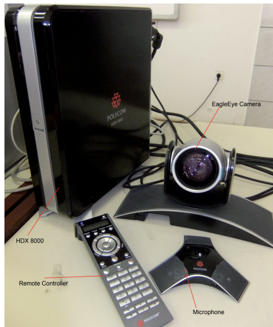
Figure 1. Polycom end conferencing equipment – HDX 8000 end point, EagleEye Camera, Remote Control and Microphone
