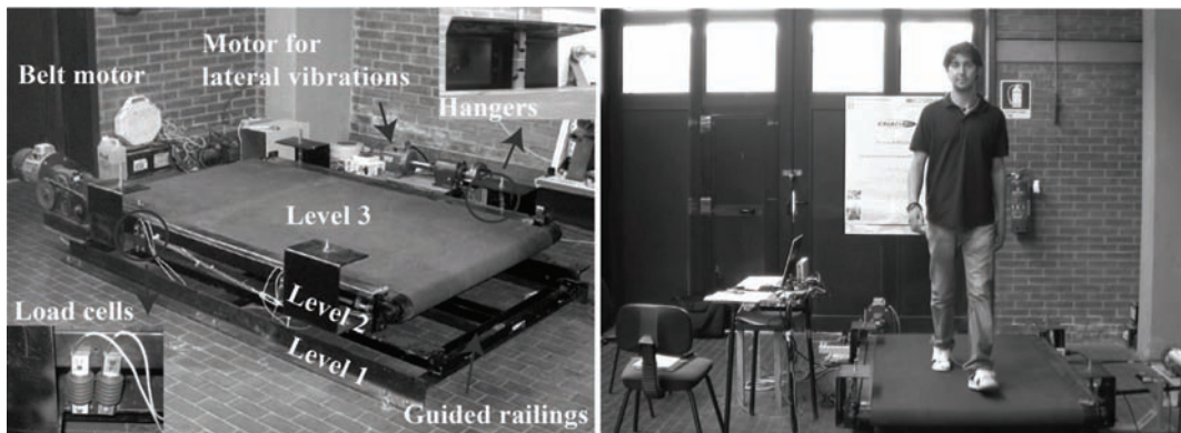
Figure 5.10 TED setup (left) and pedestrian walking test in progress (right)
