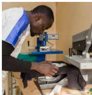
Fig. 76 Nourou places a piece of heat-film design element on a T-shirt before pressing it, 2017
