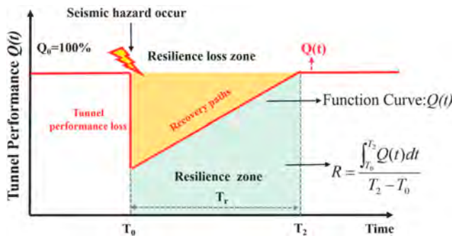
Figure 2. Definition of resilience concept for tunnel.
