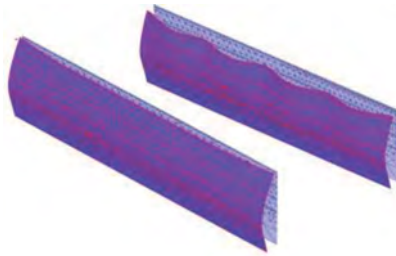
Figure 9. Deflected shape of the retaining wall (a) Conventional strut and waler system (b) PWS system.
