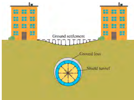
Figure 1. Tunnelling-induced ground settlement. Figure 2. Tail grouting (Liu et al., 2023).
