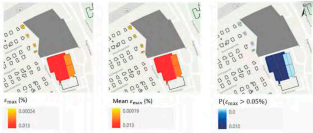
Figure 1. Excavation-induced deformations: (left) deterministic and (middle) mean maximum principal strain; probability of maximum principal strain greater than 0.05% (Zhao et al.).
