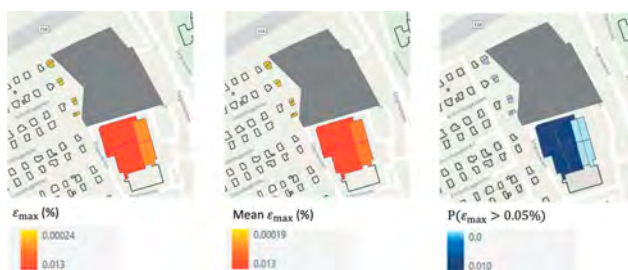
Figure 4. Second-stage assessment results. Left: The maximum principal strain ( \epsilon_{max} ) predicted with the deterministic approach. Middle: The mean of maximum principal strain ( \epsilon_{max} ) predicted with the PPBA approach. Right: The probability of maximum principal strain greater than 0.05% ( P(\epsilon_{max} > 0.05\%) ) predicted with the PPBA approach.
