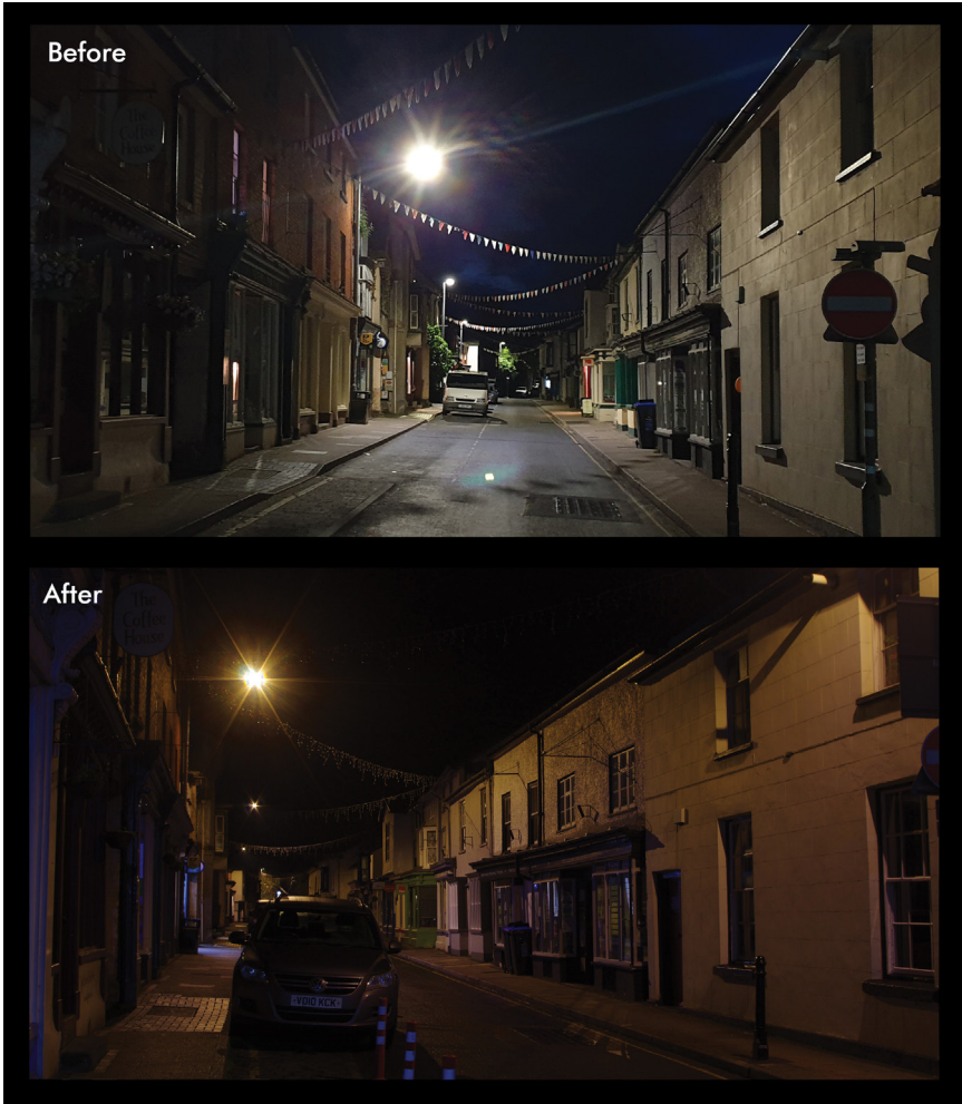
Figure 11.2 Images show the impact of replacing the white cool LEDs with warm white bulbs in Presteigne, Powys, Wales. Photo by Leigh Harling Bowen.
