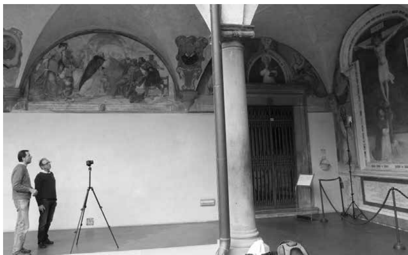
Fig. 5 VNIR hyperspectral camera during measurements in the Sant'Antonino cloister at the Museum of San Marco, Florence.
