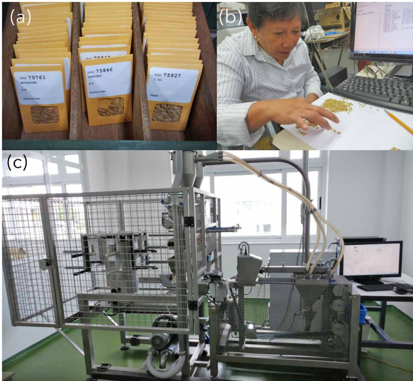
Figure 4 (a) Samples from the genebank’s physical seed file at the International Rice Research Institute (IRRI); (b) selecting the training-set seeds from the bulk prior to automated sorting (image used with permission of N. Ruaraidh Sackville Hamilton); (c) the custom seed sorter at IRRI. (a) and (c) were taken by the first author (Fiona R. Hay).
