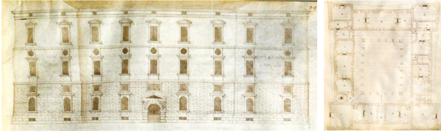
FIGURES 10.29–10.30 Serlio's plan and elevation for a fortified palace for a 'principe tiranno' in the countryside, from the Munich ms. of the Sesto Libro .
