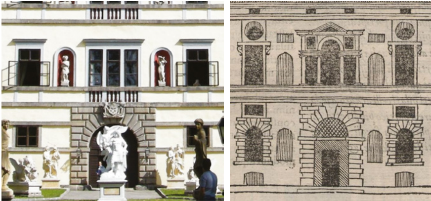
FIGURES 10.46–10.47 A detail of the entrance facade of Schwarzenau, compared to one of Serlio's proposals for the refurbishment of an old town house, in his Settimo Libro .
