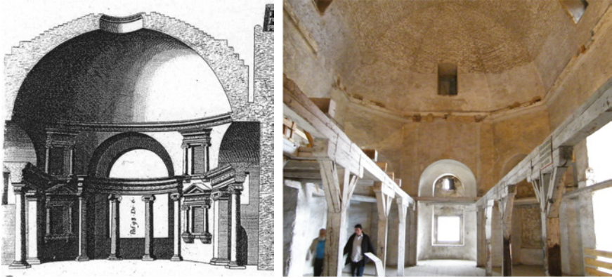
FIGURES 9.72–9.73 Section through the central rotunda of Baths of Diocletian in Rome, detail of Fig. 9.71 , compared to the hall in the West pavilion of the Neugebäude.
