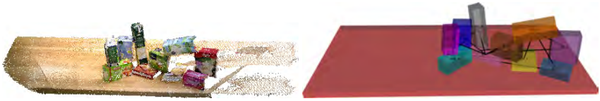
Figure 3.5: Left: Input point cloud. Right: Fitted geometric primitives and extracted support relations based on the input point cloud.
