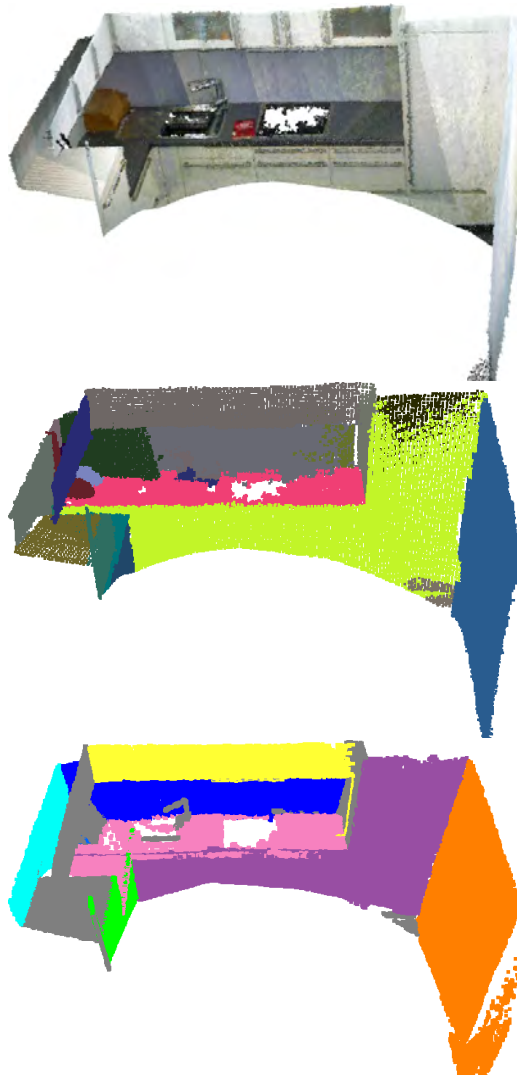
Figure 3.9: Kitchen scenario as described in Section 3.4.2. Top: The image shows the registered result of the source point cloud. Middle: Multiple views are first registered and then geometric primitives are extracted. Bottom: Primitives are extracted iteratively from consecutive frames. Figures taken from Grotz et al. (2017b) (© 2017b IEEE).
