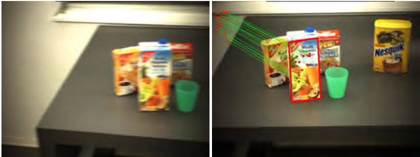
Figure 5.8: Foveal camera images during self-induced motion of the robot. Left: textured object localization without gaze stabilization, and right: textured object localization with gaze stabilization. Images taken from Grotz et al. (2017a) (© 2017a IEEE).
