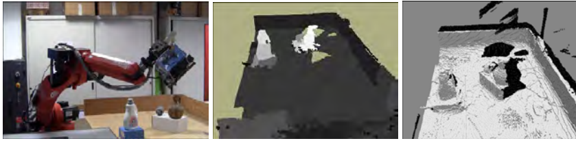
Figure 2.14: Parts of an NBV experiments. Left: the scene. Middle: saliency map of point clouds segments. Right: 3D volumetric representation. Image taken from Monica and Aleotti (2018a) (© 2018a Springer).
