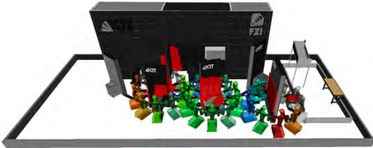
Figure 4.13: The evaluation after 6 views. The color scheme uses a heatmap to indicate the score. A low score is blue, whereas a high score is shown with a red color. Unreachable views are shown in grey.
