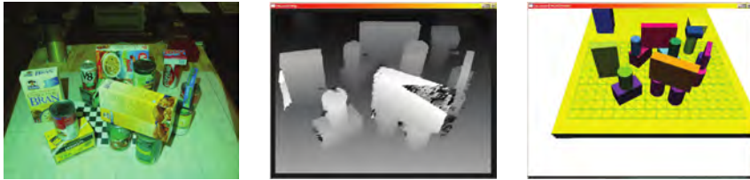
Figure 2.7: Experimental results of Hager and Wegbreit (2011) (© 2011 Sage). The scene is captured with a stereo camera system and decomposed into parametric geometric models. Left: the scene comprising of 17 objects. Middle: the disparity image. Right: the resulting scene model.
