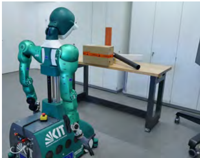
Figure 4.1: A table-top scenario. The robot cannot perceive the scene completely from the initial view due to occlusion. The robot has to change the position in order to extract a complete representation of the scene. Left: External view showing ARMAR-6 at the initial position before exploring the scene. Right: The semantic scene representation extracted from the initial view with occlusion. The semantic scene representation comprises of fitted geometric primitives and support relations in the scene. The contact points between objects, however, are not visible from the initial view.
