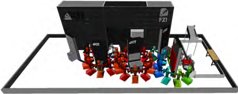
Figure 4.10: The initial view. Possible next-best-views are indicated with robot silhouettes. The color scheme uses a heatmap to indicate the score. A low score is blue, whereas a high score is shown with a red color. Unreachable views are shown in gray.
