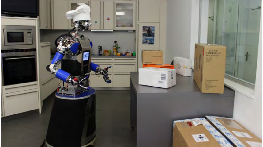
Figure 3.3: The humanoid robot ARMAR-III in a kitchen environment. The robot does not have any knowledge about the scene. The goal of the experiment is to lift a box from the table. Since both sides of the box are required for executing the manipulation action more than one view is required. Hence, multiple-views are registered with respect to each other and the geometric primitives are fitted.
