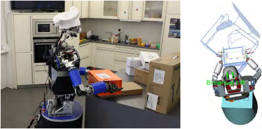
Figure 3.6: An executed bimanual lift affordance for the humanoid robot ARMAR-III. Left: An external view of the experiment. Right: Geometric primitives and extracted affordances are visualized and selected by an operator. Figure taken from the experiment of Grotz et al. (2017b) (© 2017b IEEE).
