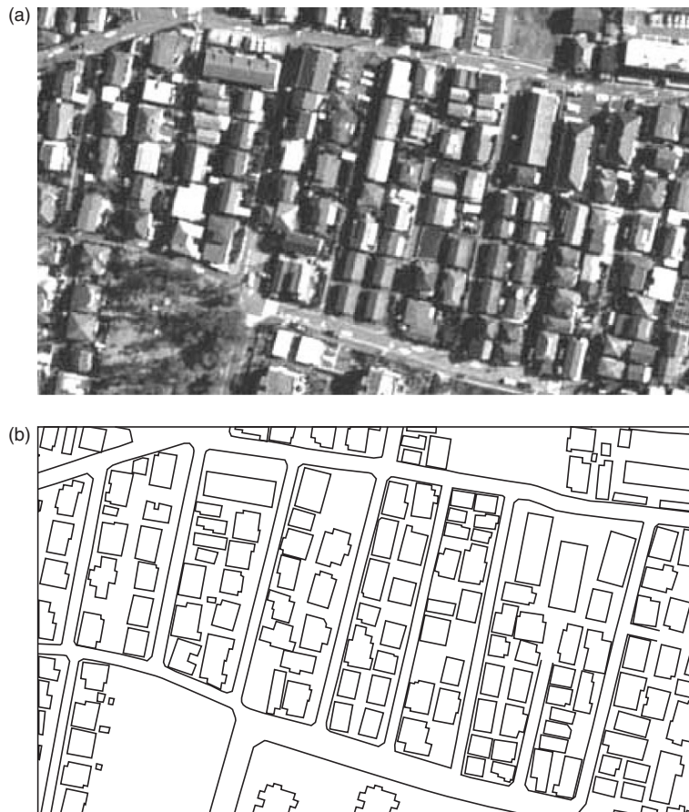
Figure 3.2 Digitization of an aerial photograph. (a) The aerial photograph and (b) the spatial data.
