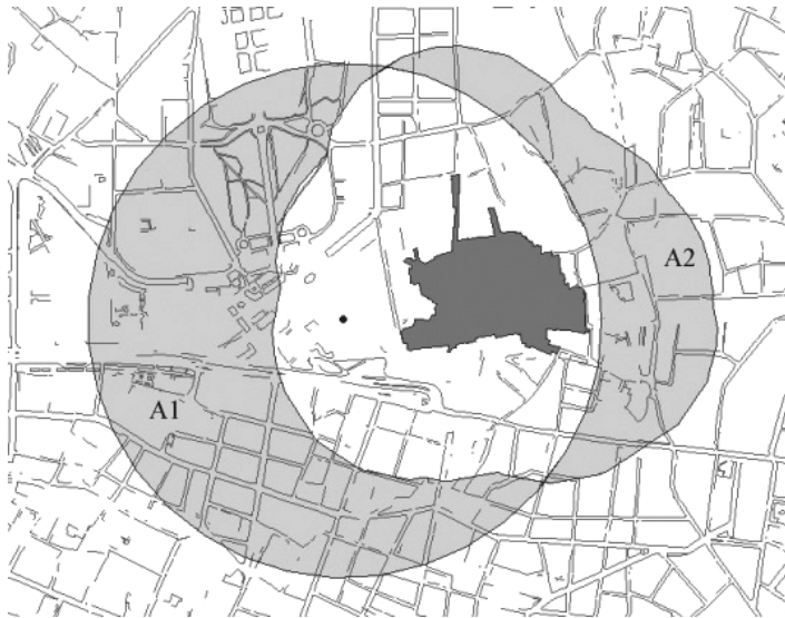
Figure 1.17 An XOR operation, A1 \text{ XOR } A2 .
