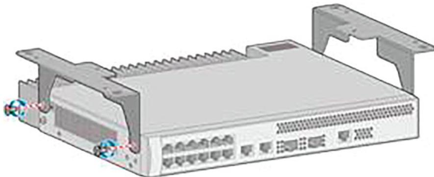
**Fig. 3.69** Installation method of the ceiling-mounting ears
