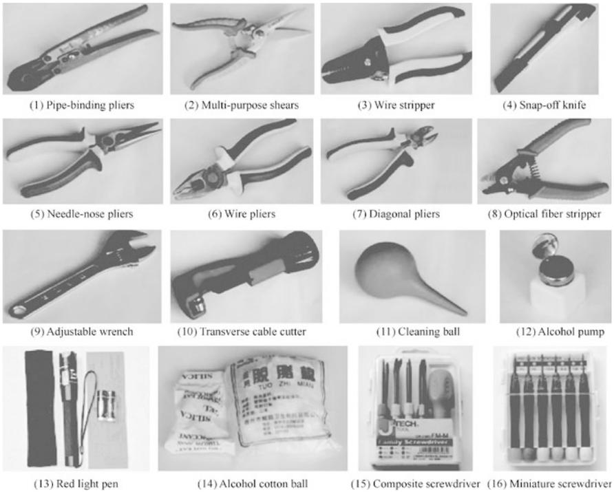
Fig. 2.49 Tools in the Xiyuan optical fiber toolbox
