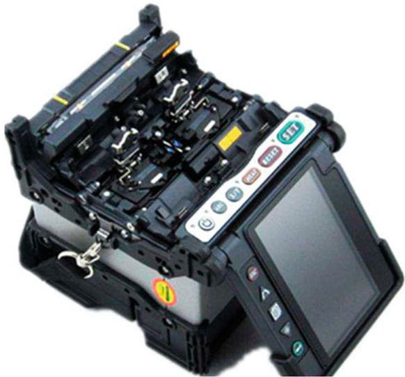
**Fig. 2.58** Toolbox of optical fiber fusion splicer
