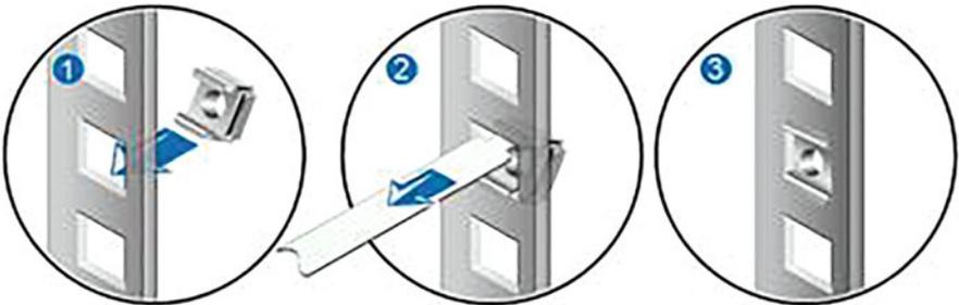
**Fig. 3.105** Install the floating nut matched with the M6 screw
