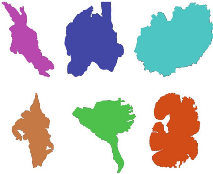
Fig. 9.1 Hydraulic fracture morphology retained by injecting fluid into the particulate material matrix
