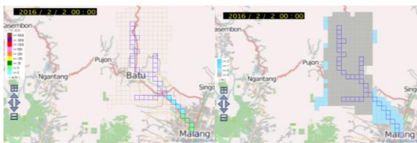
Fig. 4. RRI Model result showing the spatial simulated runoff (left) and inundation (right).
