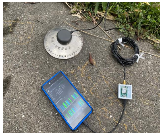
Fig. 3. Rover station of this study. RTK-GNSS receiver (NEO-M8P-0) is in a small white box in right side and Rtkgps+ (an application for RTK) on a smartphone is processing FIX data of precise positioning data.
