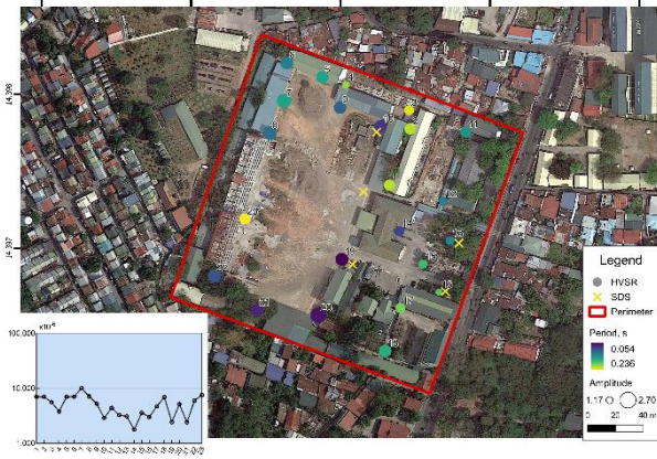
Fig. 4. Distribution of predominant period, relative amplitude, and seismic shear strain in TNCHS. Also shown are the locations of SDS boreholes.
