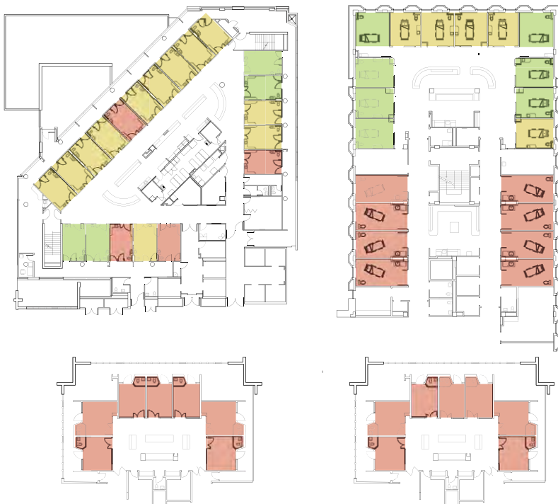
2.7 High (green), medium (gold) and low (red) isovist connectivity values for patient rooms in four ICUs. Image by Victor Carrillo and Daniel Rios, 2021.
