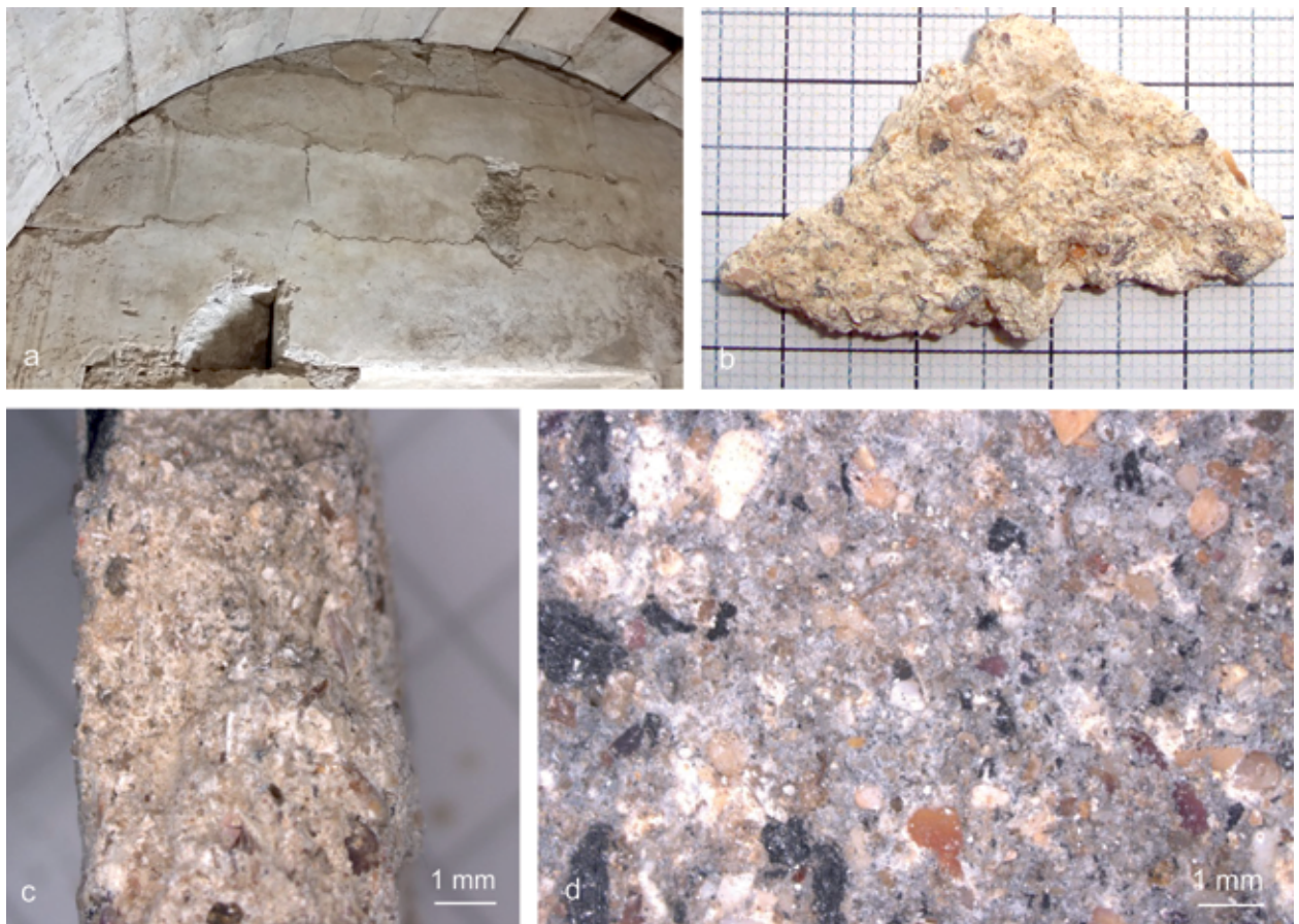
Figure 157. a) Eastern wall of the funerary chamber; b) fragment of brownish-whitish mortar, in which the quartz granules from translucent to yellowish and grey are clearly observable, their edges being rounded to subangular; sorting is medium to weak in the size range 0.5 mm - 3 mm, but uniform overall; c) the thickness of the level of mortar with plaster does not exceed 5 mm - 8 mm; c) although less than 1 cm thick, the mortar was deposited in several successive levels, of which the base is obviously coarser and of a greyer shade, followed by a slightly finer subcentimetric level and an obviously smoother and better final layer. The main compounds are carbonatic clasts, fossiliferous remains, tabular-prismatic granules of crushed coal, but also granules from subangular to sub-rounded white, grey, brown or brick translucent quartz, in varying degrees of opacity; d). the grey layer of mortar includes angular to subrounded psamitic size clasts in a carbonatic binder; the grey colour is due to large to small fragments of charcoal.
