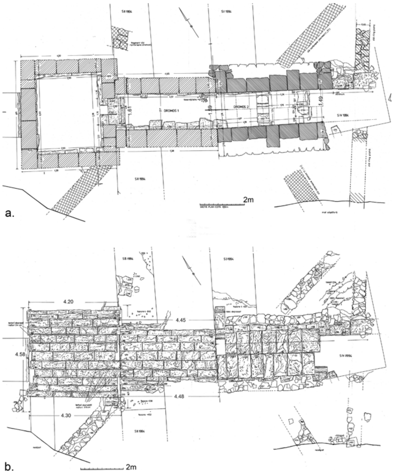
Figure 94. Drawings by the architect Anișoara Sion (1999: pl. III, IV), based on measurements (by hand and with alidade) from 1993-1994. Even if the more recent digital documentation activity in the tomb revealed a variety of differences between the tomb's interior and Sion's documentation – e.g. in block dimensioning and the numbers per row (as the plaster fell away over time, revealing the joints more clearly), or in the general angles of the compartments – these drawings are especially valuable for the extrados recording, which has never again been uncovered since. The section (a) was made along the third masonry row (numbered from bottom up).
