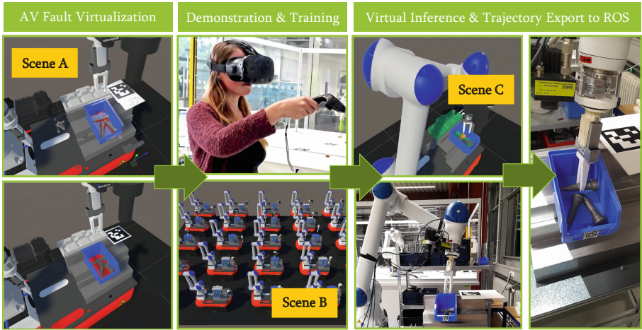
Fig. 3. Evaluation workflow involving AV fault virtualization, demonstration and training as well as virtual inference and ROS-trajectory export; in addition: real-world bin picking setup with exemplary grasping component “shifting rod” and YASKAWA HC10 articulated robot.
