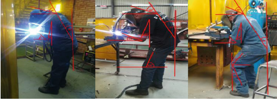
Fig. 1. Postural configuration of the welders with body physique dimensions within the 5 th , 50 th and 95 th percentile
