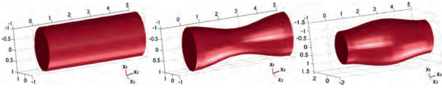
Figure 6.10: Reference pipe and two deformed pipes ( \mu = -5, \mu = 5 ): stenosis and aneurysm configurations.
