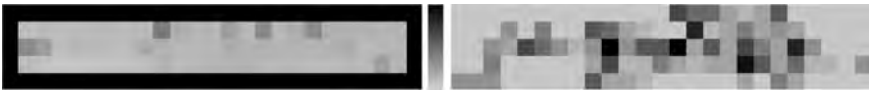
Figure 6.8: Spatial distribution of the final sizes of the local reduced bases on each subdomain, after the adaptive online phase for the experiment in Section 6.8.1 with \Omega = [0, 5] \times [0, 1] , |\mathcal{T}_H| = 25 \times 5 for the two strategies shown in Figure 6.7: no global snapshot with uniform enrichment (left, light: 24, dark: 148) and two global snapshots with adaptive enrichment (right, light: 9, dark: 20). Note the pronounced structure (right) reflecting the spatial structure of the data functions (compare Figure 6.6).
