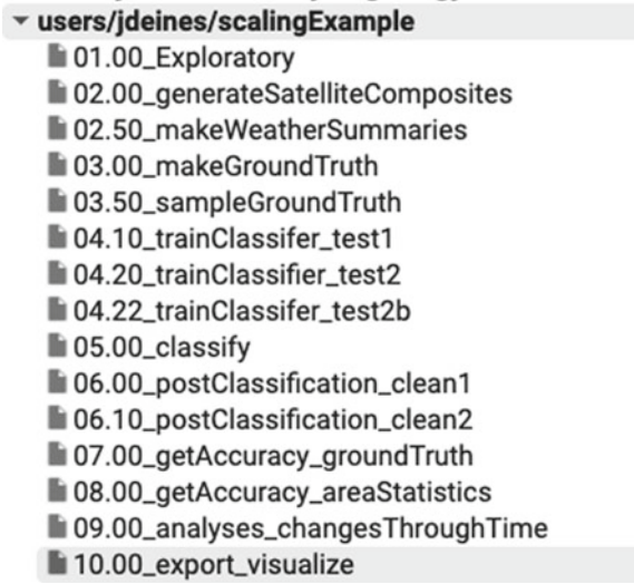
Fig. 29.13 Example project repository with multiple scripts. Using leading numbers when naming scripts allows you to order them by their position in the workflow
