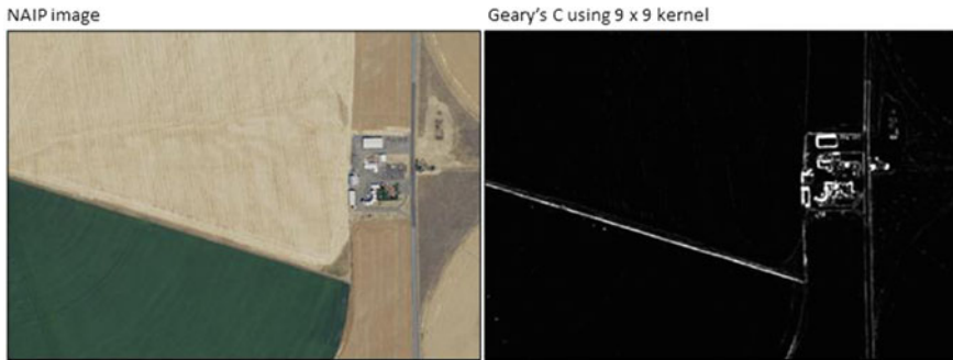
Fig. 10.16 Example of Geary's C for the NAIP imagery using a 9 m kernel
