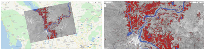
Fig. 42.10 Extracted flood areas by comparing the calculated surface water map against the JRC permanent water data. Bottom image shows a close-up of the flood map around the confluence of the Mekong and Tonle Sap rivers near Phnom Penh, Cambodia
