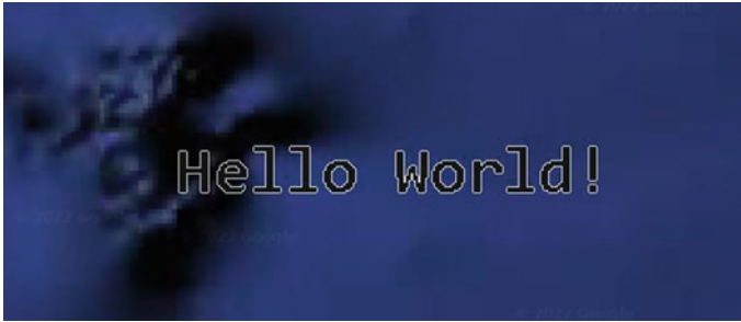
Fig. 27.8 Rendering text with adjusted parameters (font type: Consolas, fontSize: 32, textColor: 'black', outlineWidth: 1, outlineColor: 'white', outlineOpacity: 0.8)
