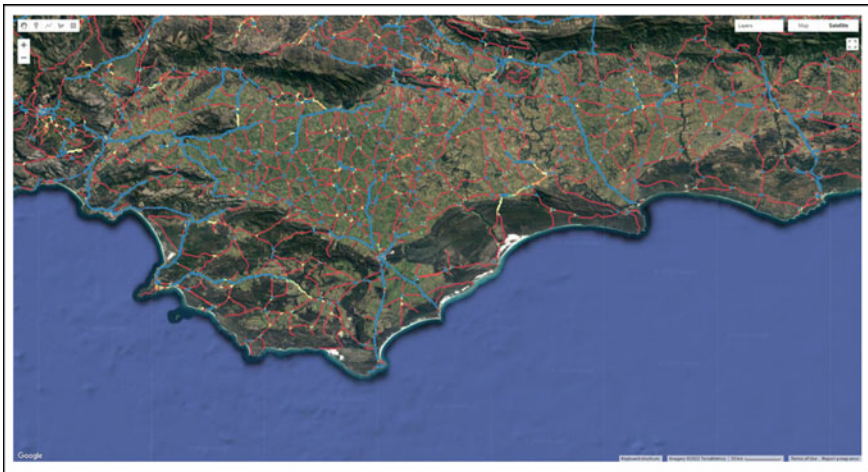
Fig. 34.3 Results of Geary's C^* spatial autocorrelation between roads and transmission lines in South Africa. Red indicates clustering, while blue indicates dispersion. Shorter stretches in this example appear to have more co-located linear infrastructure
