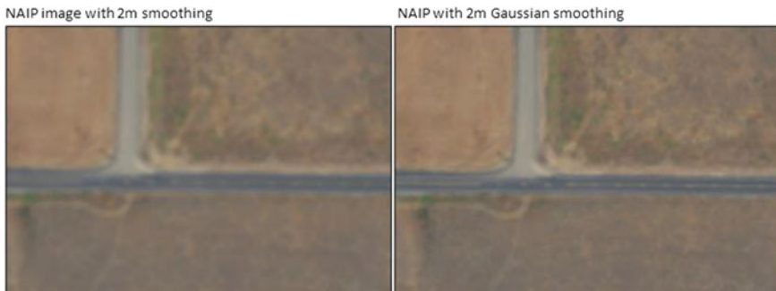
Fig. 10.3 Example of the effects of a Gaussian smoothing kernel on NAIP imagery using a 2 m kernel
