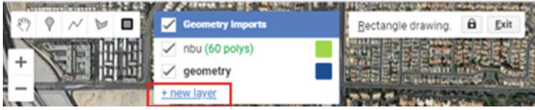
Fig. 33.10 Creating a new layer for the built-up FeatureCollection To create a new empty feature collection of built-up examples, click on the + new layer (at the bottom of the Geometry Imports )
