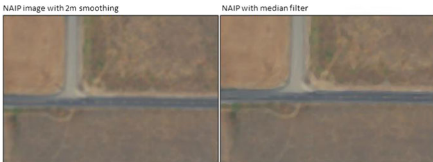
Fig. 10.6 Example of the effects of a median neighborhood filter on NAIP imagery
