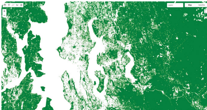
Fig. 5.7 Thresholded forest and non-forest image based on NDVI for Seattle, Washington, USA
