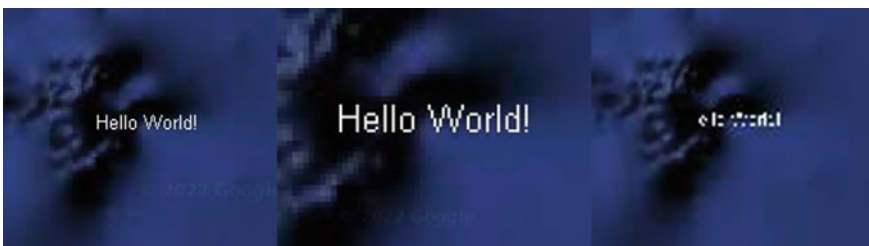
Fig. 27.7 Results of the text.draw call, scaled to 1x: var scale = Map.getScale() * 1 (left); 2x: var scale = Map.getScale() * 2 (center); and 0.5x: var scale = Map.getScale() * 0.5 (right)
