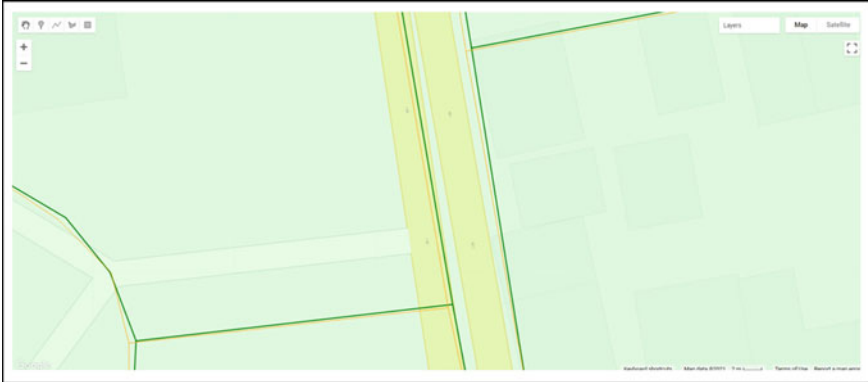
Fig. 34.2 Examining roads from the GRIP dataset as features (in green) versus rasters (in orange) overlaid with transparency on the Map view. There can be offset between datasets and different spatial shapes (lines, polygons, and rasters)
