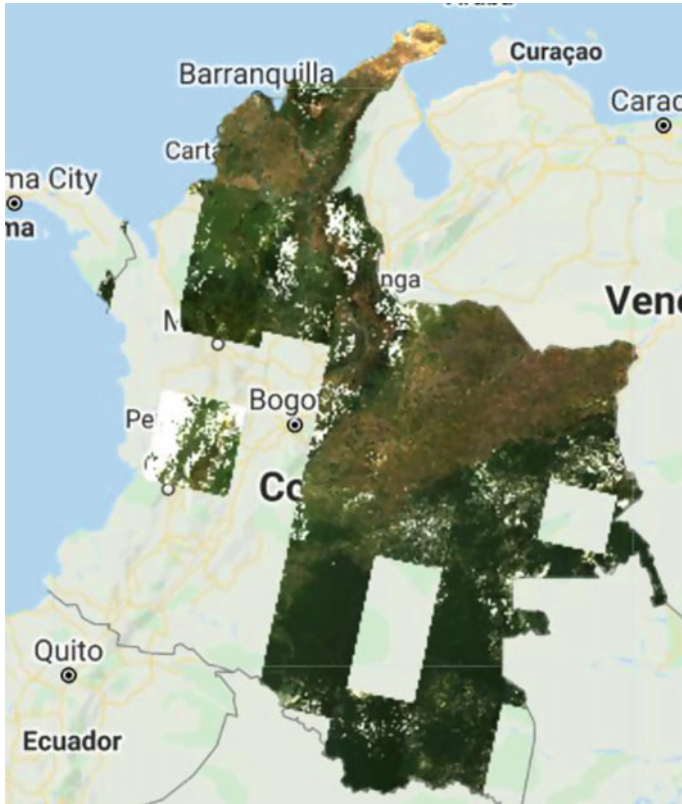
Fig. 15.3 Landsat 8 surface reflectance 2019 median composite of Colombia filtered by cloud cover less than 20%
