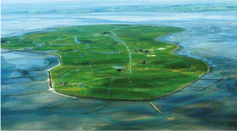
Figure 4.2 Aerial view of Hallig Hooge with the island of Pellworm at the horizon. On Hooge, about 100 people live on dwelling mounds (Warften). A salt marsh area of 5.5 km 2 is inundated by storm surges which top a 1.2-metre-high stone revetment. Sediment accretion is now lagging behind sea level rise because of the revetment.
