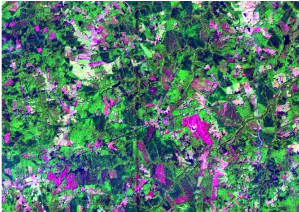
Fig. 7(a). Zoomed area of a Landsat 7 ETM+ image of Virginia, USA (path: 16, row: 34, acquisition date: 2002-09-13), depicted in false colors (R: band ETM5, G: band ETM4, B: band ETM1), 30 m resolution, calibrated into TOARF values.
