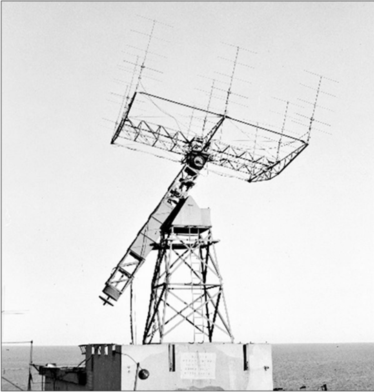
Fig. 4.10 The 9-Yagi array on its equatorial mounting was used to carry out the first survey of the southern sky at 100 MHz (after Pawsey and Bracewell, 1955: Plate 2)
