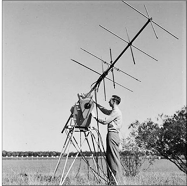
Fig. 2.39 Joe Pawsey with one of the 97 MHz Yagi antennas used with the three-element position interferometer. The crossed dipoles allowed the polarisation of the solar bursts to be determined (courtesy: Life magazine)
