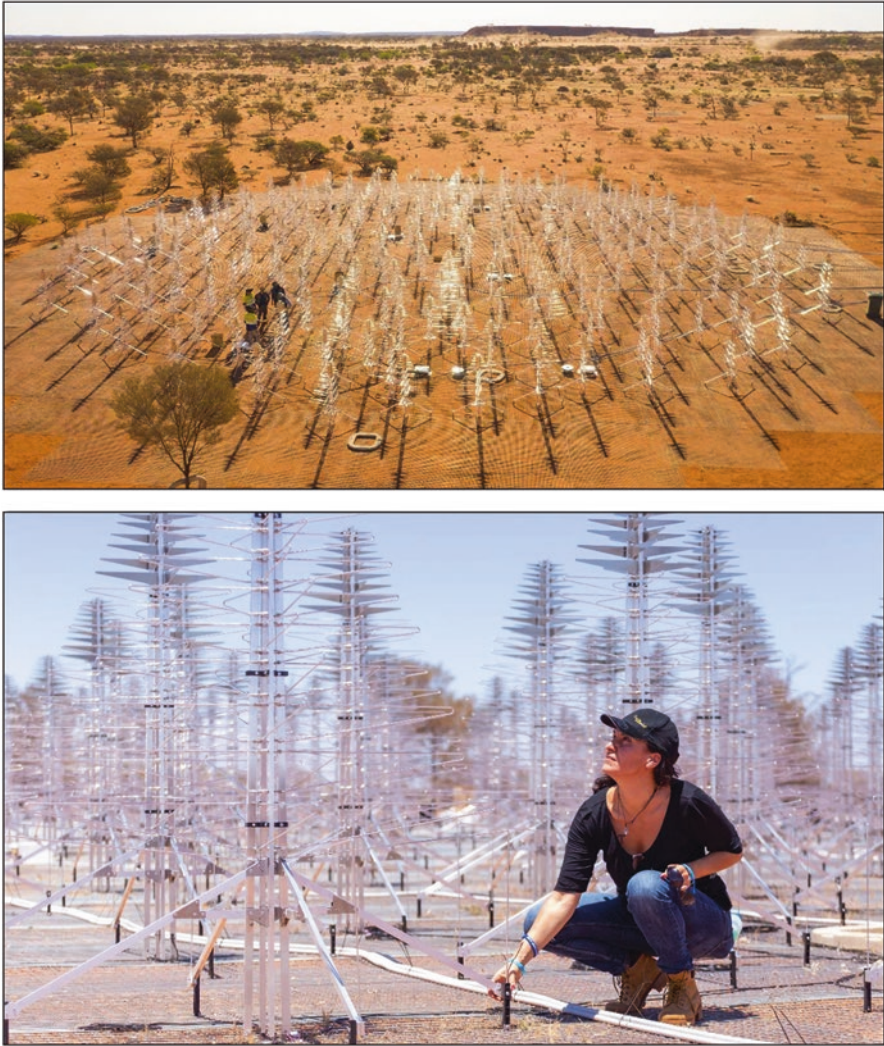
Fig. 5.29 (above) The Aperture Array Verification System (AAVS) is a testbed for optimising the design of the SKA-Low antennas. (below) SKA-Low engineer Maria Grazia Labate inspects one of the 256 ‘Christmas tree’ antennas making up the AAVS. The antennas have been designed to minimise cost and to maximise reliability in their harsh climate (courtesy: ICRAR/Curtin University)
