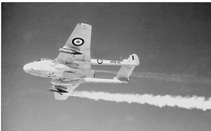
Fig. 1.12 During the 1950s and 1960s, apart from radio astronomy, the other major research area at Radiophysics was rainmaking. Silver iodide burners were attached to aircraft and used to seed clouds in selected areas of eastern Australia. Military aircraft were used for the trials because silver iodide is highly inflammable and too dangerous to use on commercial aircraft (courtesy: CRAIA)
