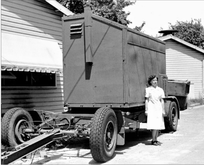
Fig. 2.15 The ex-Army radar trailer in the grounds of the Radiophysics Lab, shortly before it was shipped to Auckland, New Zealand. This mobile sea interferometer featured four Yagi aerials, a new 100 MHz receiver, recorders, chronometers, weather recording instruments and all the tools and backup equipment needed to operate reliably at a remote location (courtesy: CRAIA)
