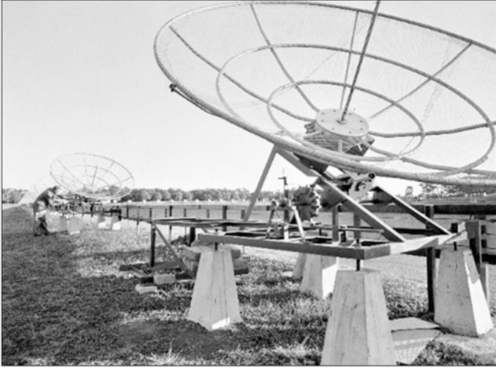
Fig. 2.41 The 16-element north–south arm of the solar grating array in July 1953, located on the eastern bank of the Potts Hill reservoir. The E–W arm can be seen in the background on the southern bank (courtesy: CRAIA)
