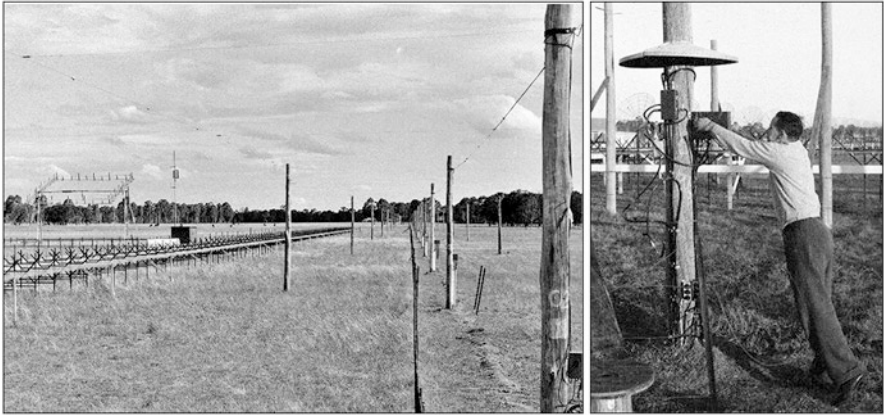
Fig. 2.63 (left) Section of the 19.7 MHz Shain Cross at Fleurs, also showing part of the N–S arm of the Mills Cross and the broadside array used for long baseline interferometry. (right) Alex Shain making adjustments to one of the dipole phase switches located along the N–S arm of the Shain Cross. The switches allow the beam to be directed to different E–W positions (courtesy: CRAIA)
