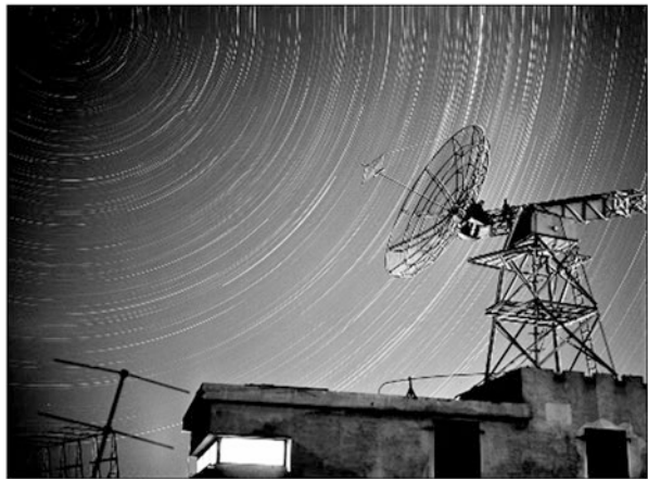
Fig. 2.19 Star trails and the 3.9 m parabolic dish on the roof of the Dover Heights blockhouse (courtesy: CRAIA)
