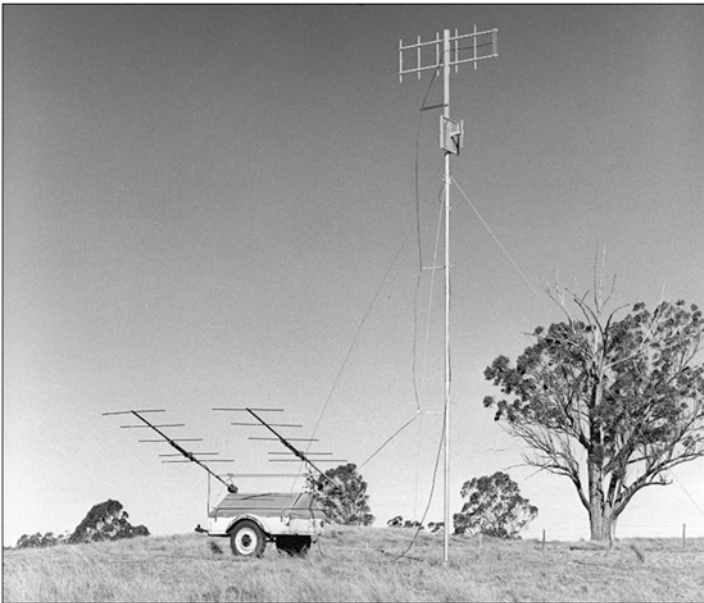
Fig. 2.55 The mobile two-element Yagi array and microwave link formed part of the variable baseline interferometer at Badgery's Creek. This array was used in conjunction with the broadside arrays to study four of the brightest discrete sources at 101 MHz (courtesy: CRAIA)
