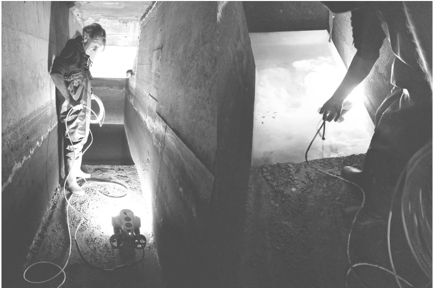
Figure 6.14: Only known entrance to the basement in the eastern section of the bunker. Images show the poor illumination conditions, narrow access, and level of flooding in the basement, as well as the Remote Operating Vehicle (ROV) used for exploration.
