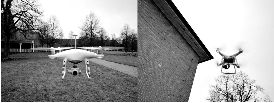
Figure 6.11: Micro Aerial Vehicle (MAV)—DJI Phantom 4 Pro v2.0—used to record the bunker outdoors.
