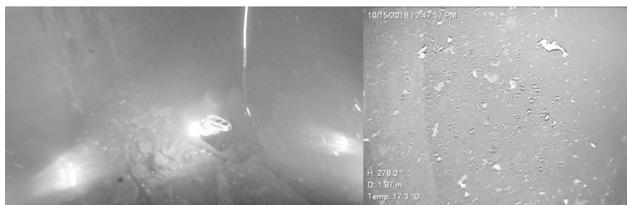
Figure 6.16: (Left) view of the Remote Operating Vehicle exploring a water basin with clear water; (right) example of sediment particles hindering camera vision through light backscatter.
