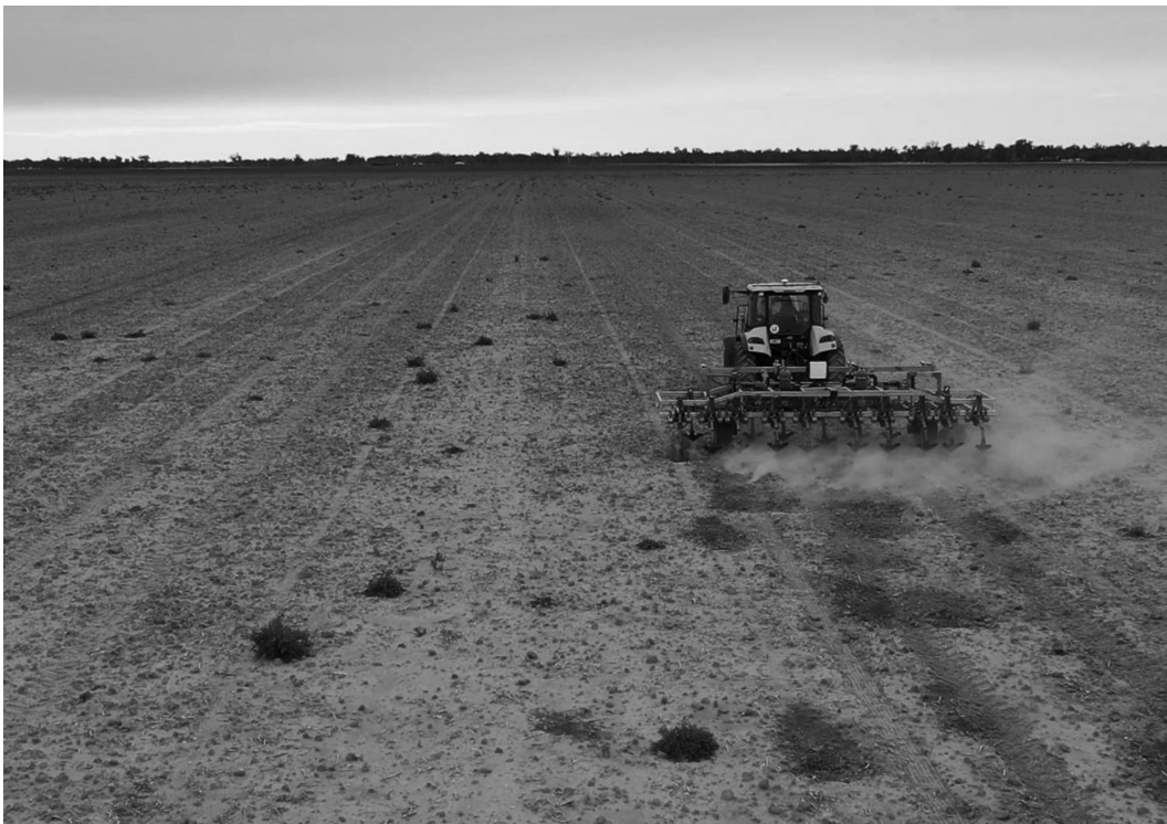
FIGURE 11.5 The Weed Chipper in operation in a fallow field in NSW. The tynes which are held in a stand-by position above ground are triggered by cameras to chip out weeds.
