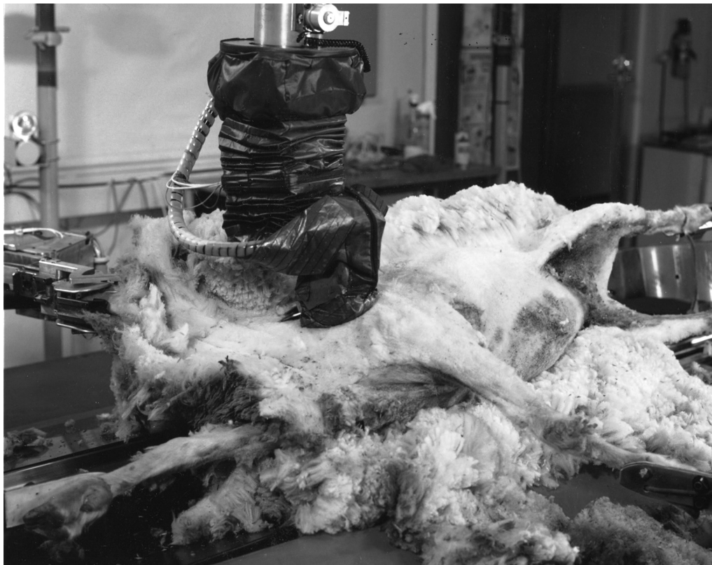
FIGURE 11.4 Robotic sheep shearing, 1989. The team tapped the expertise of human shearers to improve the robot's performance. Video of the robot operating is available at: https://www.youtube.com/watch?reload=9&v=6ZAh2zv7TMM
