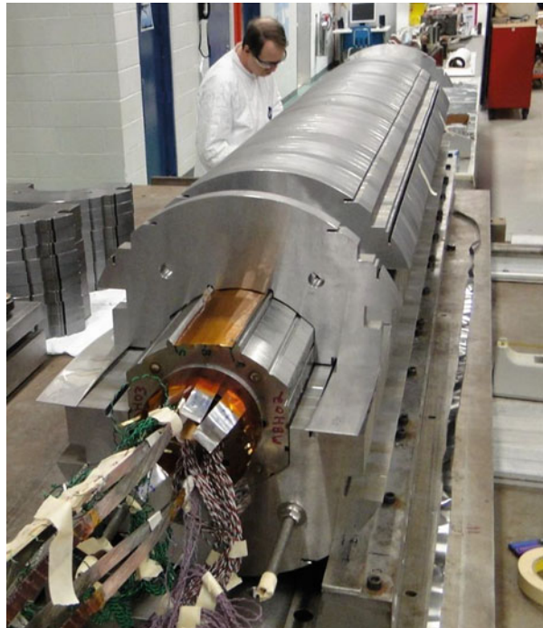
Fig. 8.10 Collared coil with collar-yoke shims inside iron yoke (lead end)
