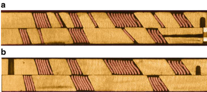
Fig. 6.11 A longitudinal cut through (a) the inner coil lead-end; and (b) the return-end (compare with Fig. 6.7)
