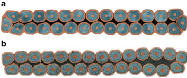
Fig. 7.12 Cross-sections of (a) 28-strand and (b) 27-strand cables
