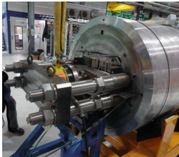
Fig. 12.14 Magnet after coil-pack insertion. The picture shows the elements of the assembly
