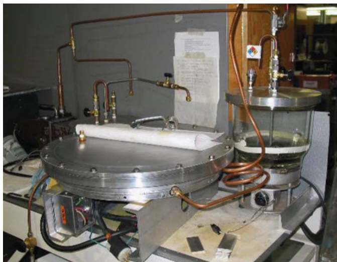
Fig. 14.12 Vacuum-impregnation fixture for coating cable with Mobil-1 ® to avoid sintering
