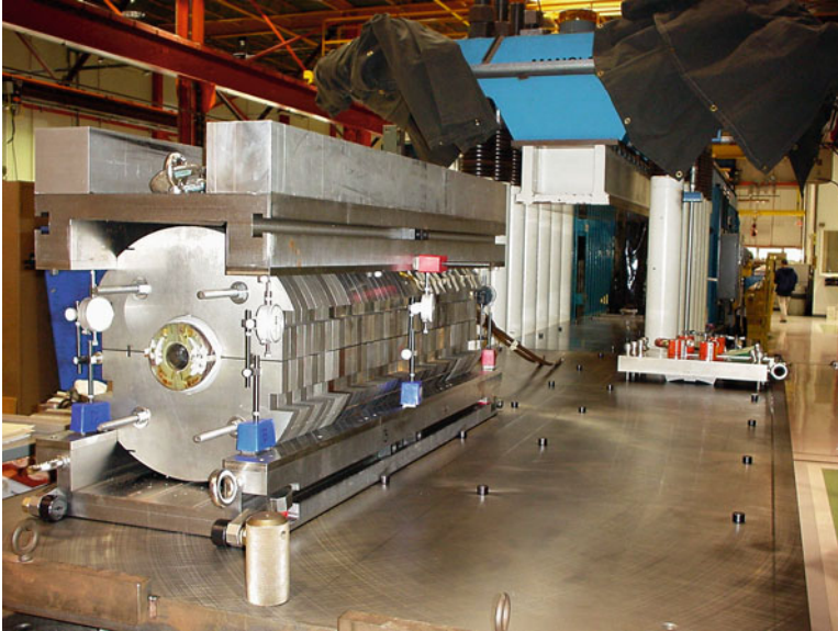
Fig. 7.10 Coil-yoke assembly inside the yoking and clamping tooling ready for installation in the vertical press. (Chichili et al. 2001)
