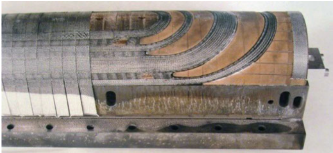
Fig. 6.10 Prototype coil with tape insulation added (note the carbon residue)
