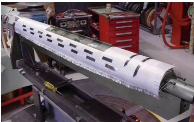
Fig. 7.7 The middle layer of the inter-layer insulation with strip-heaters. (Chichili et al. 2001)
