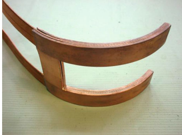
Fig. 15.11 The copper-stabilized pre-formed splice
