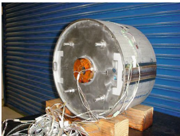
Fig. 7.6 Instrumented short mechanical model. (Andreev et al. 2000)
