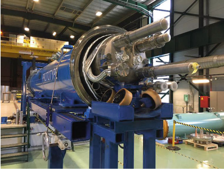
Fig. 9.17 The first 5.5 m long 11 T MBH dipole prototype in its cryostat at CERN ready to be transported to the test bench
