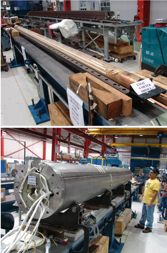
Fig. 7.23 (a) First in the world 4 m long Nb_3Sn dipole coil. (b) Dipole mirror LM02 with 4 m coil prepared for transportation to the FNAL magnet test facility. (Zlobin 2011)
