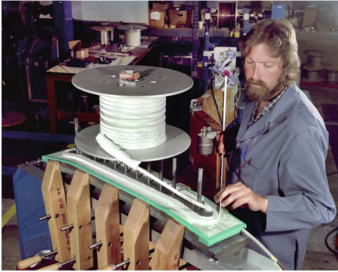
Fig. 11.9 Roy Hannaford winding the D10 coils (ca. 1983). The flared end and inter-layer transition of HD2 closely follows the concept developed for D10
