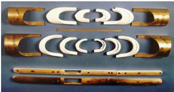
Fig. 6.8 Layers 1 and 2 pole blocks (islands), end spacers, and saddles (shoes). White alumina coating was added to the end spacers for extra insulation
