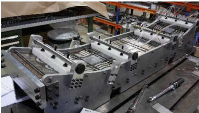
Fig. 12.12 Coils 1–2 and 3–4 installed in the tailored shim impregnation mold
