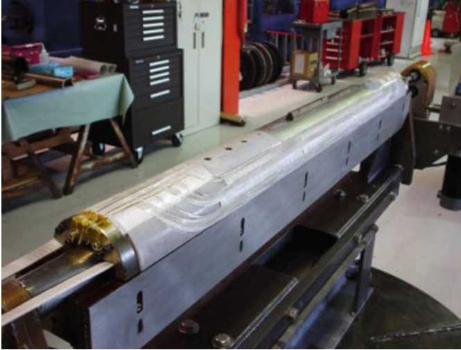
Fig. 7.8 Dipole coil with coated parts after impregnation with ceramic binder and curing in a precise mold. (Chichili et al. 2001)
