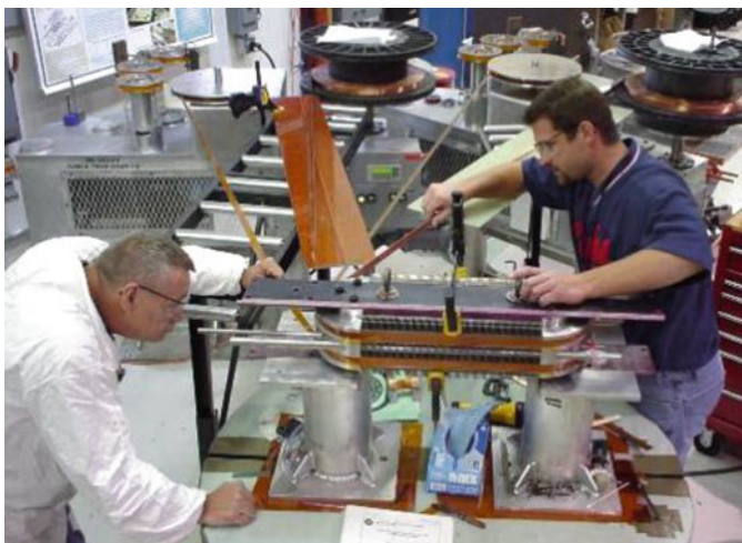
Fig. 15.13 Coil winding is performed horizontally using a rotating table. Four independent tensioners, shown in the top part of the picture, are used to apply a tension to each cable and to the insulation tapes
