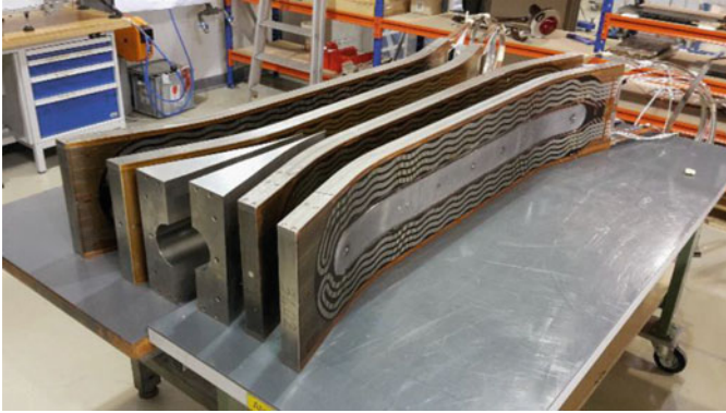
Fig. 12.11 Four Nb 3 Sn coils of one magnet are ready for the first magnet assembly
