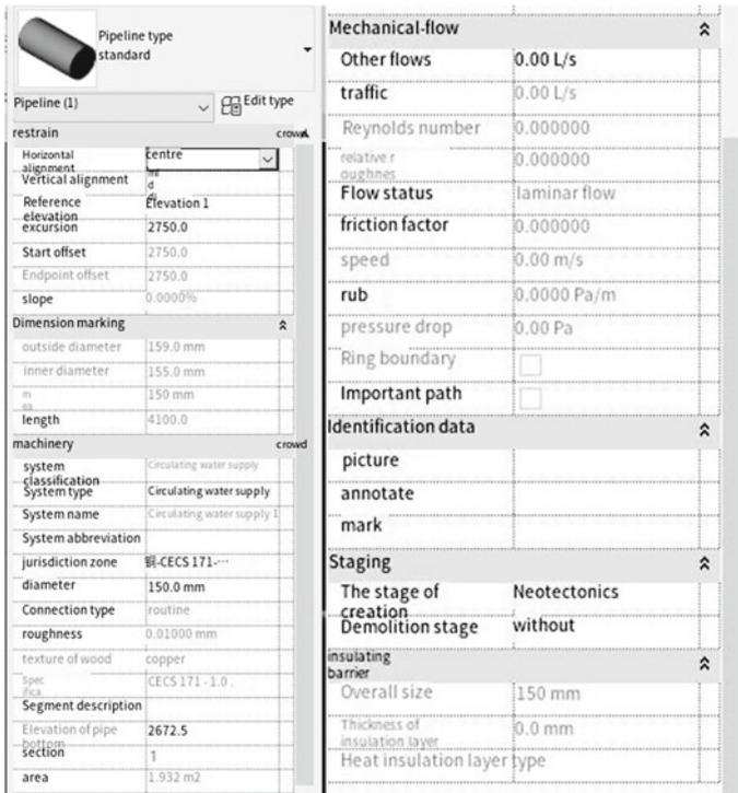
Fig. 2 Data structure of pipeline information in Revit software
