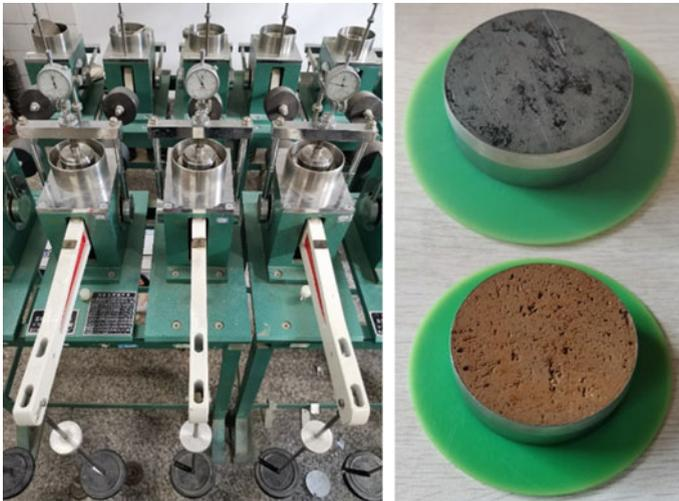
**Fig. 1** The consolidation instrument and soil samples
