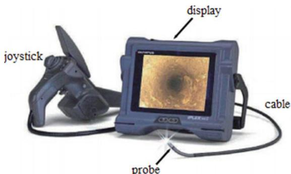
A tiny camera takes pictures of the scene under the light source, and then converts the images into digital signals that are transmitted by cable to the display screen [8].
