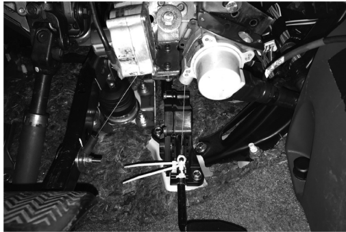
Figure 9. Example of pedal position measurement using string potentiometer. Body of device is secured to hard points under the dashboard structure.
