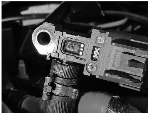
Figure 30. Vehicle A DPF sensor. The backside of the sensor package houses an ambient pressure reference that is used to determine a differential signal compared to pre-DPF pressure tapping location.
