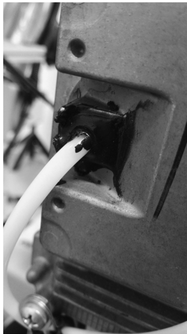
Figure 32. Vehicle A ECU is modified similar to the image above. Breather cap for detecting ambient pressure is removed and sealed with 6 mm nylon pipe inserted. Nylon pipe references to MEDAS inlet. ECU is not fully airtight but it is enough for MEDAS to maintain an pressure inside.
