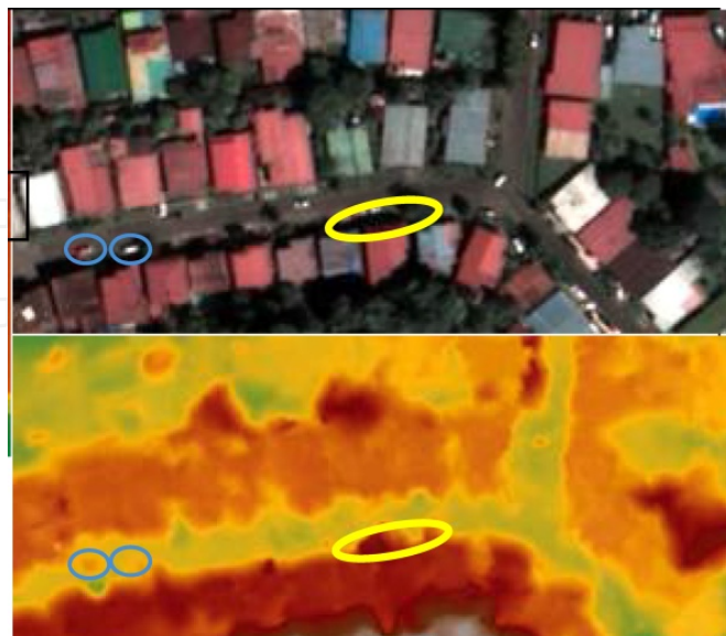
Figure 14. Example of effects of shadows and moving objects in the DEM (Panama City). Above: pansharpened nadir scene; below: DEM
