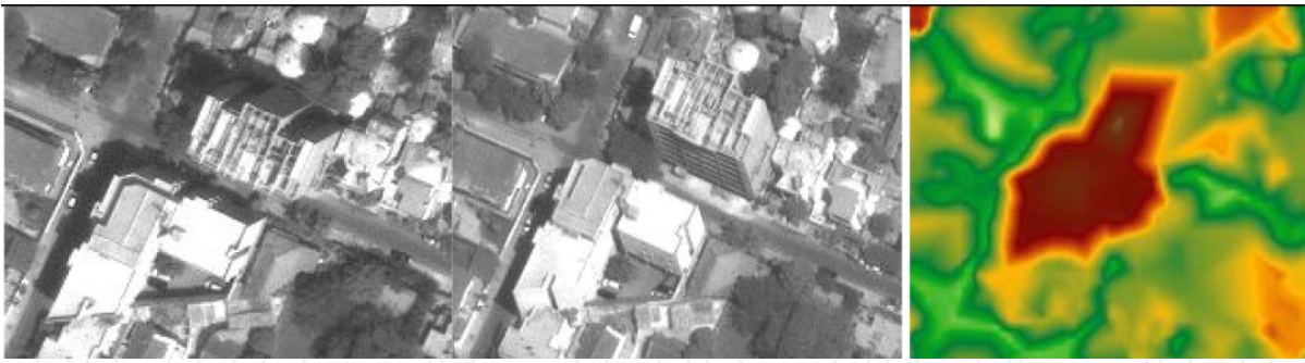
Figure 15. Example of corridor occlusion due to tall buildings; (a) and (b): stereo images; (c) resulting DEM (Dakar).
