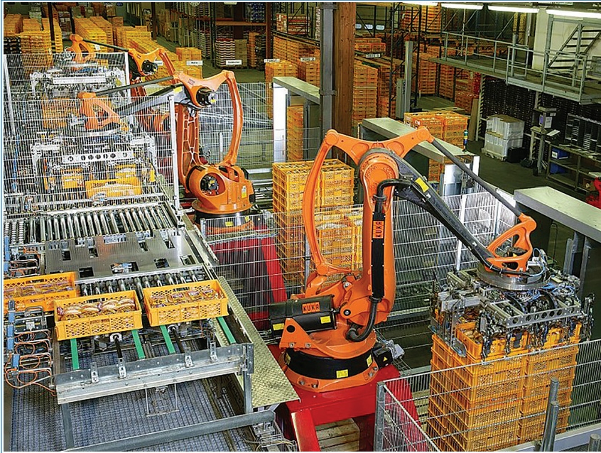
Figure 4.1. A Kuka robot palletizing food in a bakery (taken from Wikipedia).
