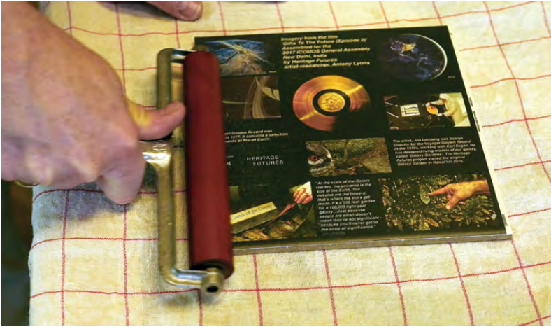
Figure 21.7 Part of the process of making the tablets: applying the ceramic print layer before kiln-firing (photograph by Antony Lyons).
