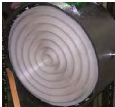
**Fig. 1:** Dummy load for HPM  $TM_{011}$  calorimeter.
