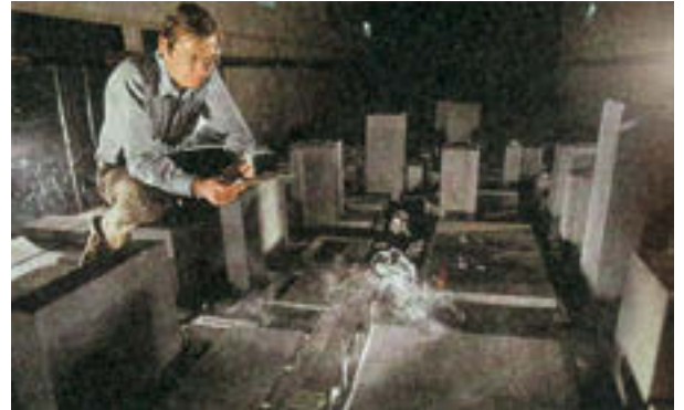
223 Smoke simula- tions in the wind tunnel, Colorado State University (USA).
