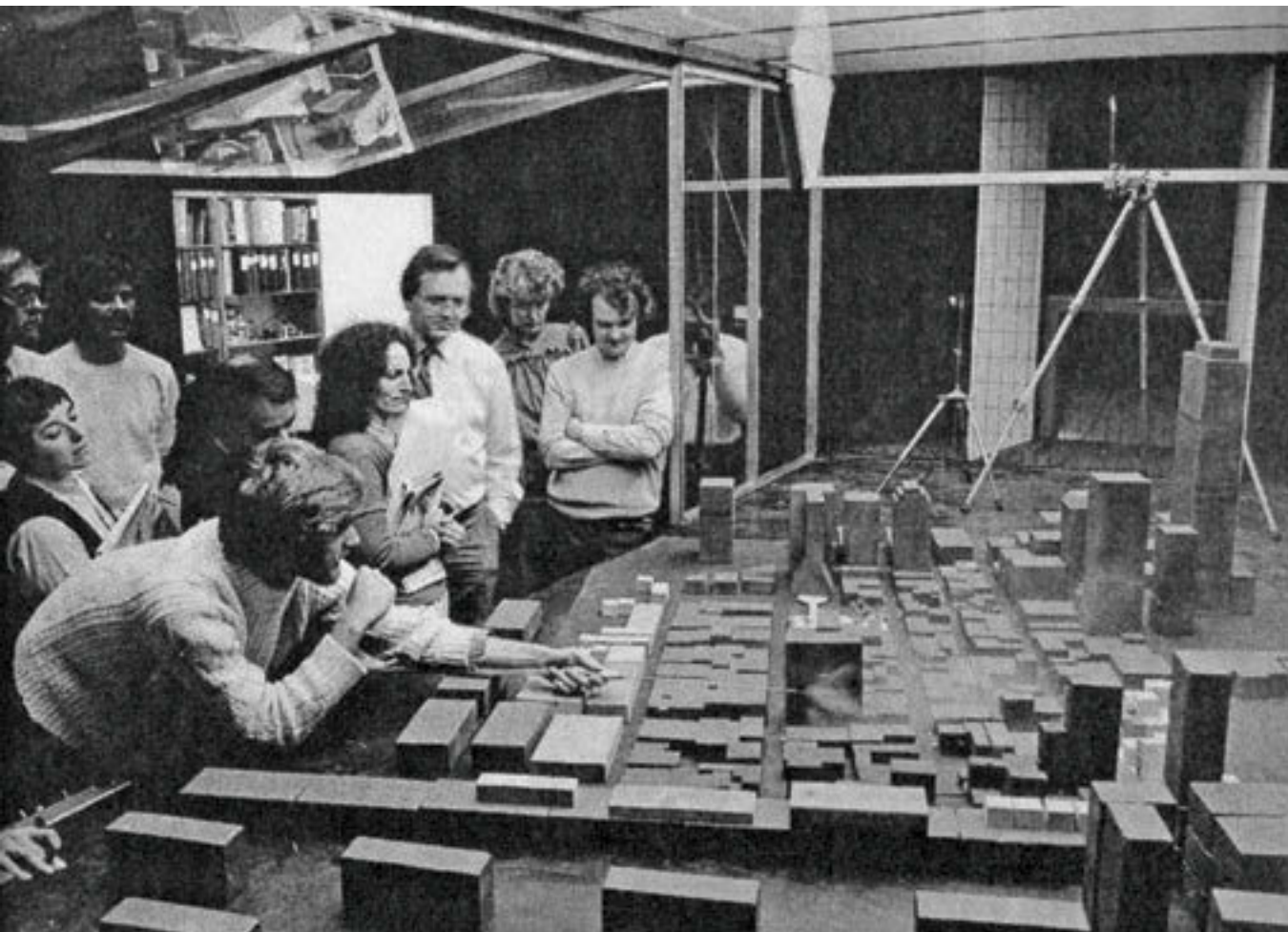
224 Exploring the wind profile of downtown San Francisco (USA). Environmental Simulation Laboratory, UC Berkeley.
