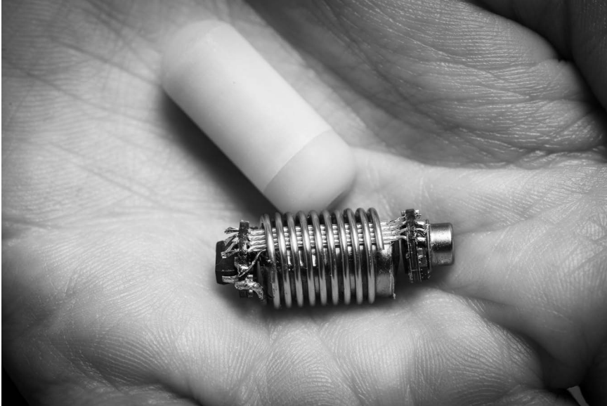
Figure 6.3 The packaged capsule (above) and the open capsule (below), showing the electronic circuit, sensors, packaged batteries and coil antennae. Photo supplied by Kourosh Kalantar-Zadeh.
