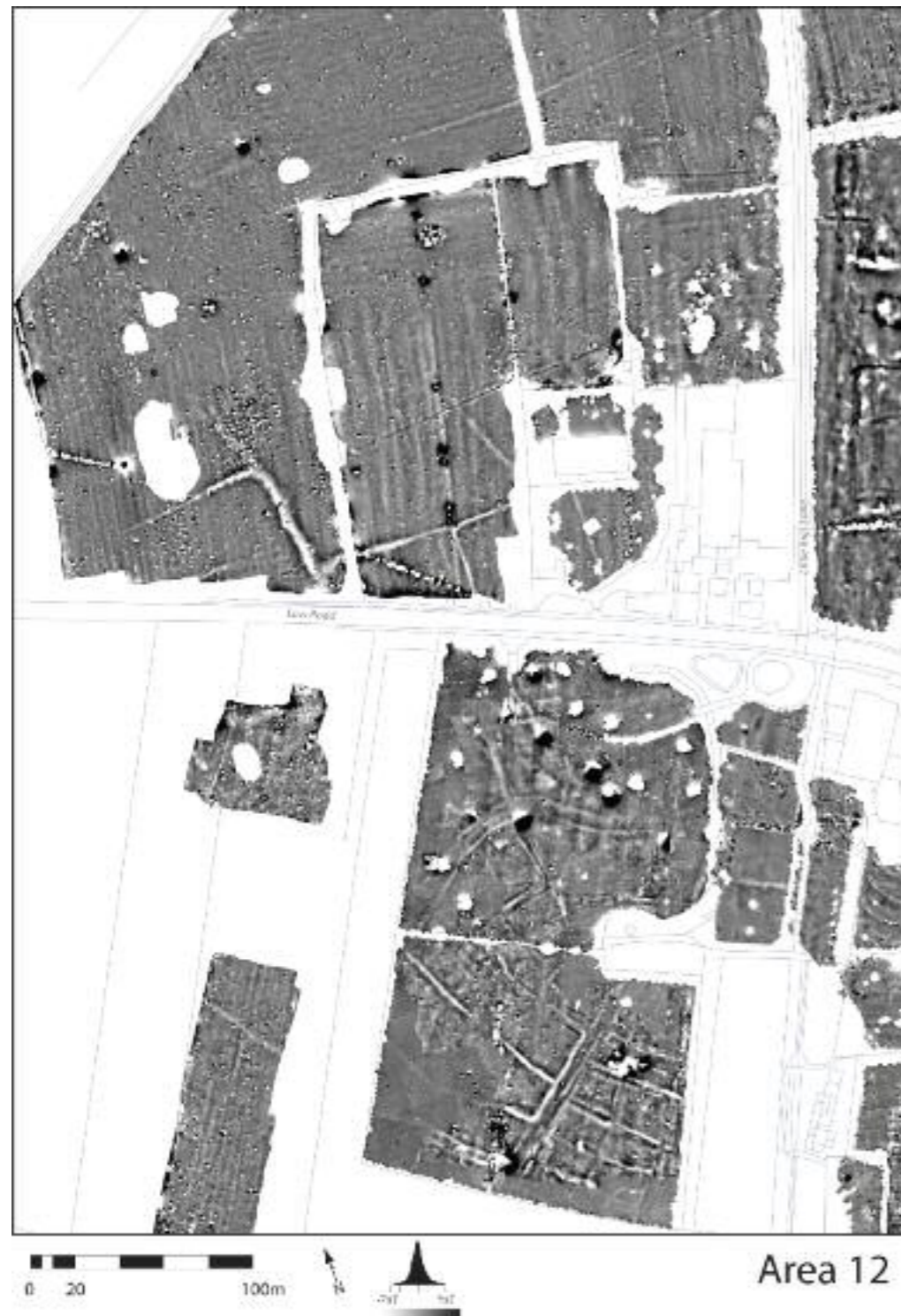
Fig 3.41 Area 12: results of the gradiometry survey in relation to modern topography. For the location, see fig 3.3. Scale 1:3000. Drawing: Rose Ferraby. © Crown copyright and database rights 2018 Ordnance Survey (100025252)
