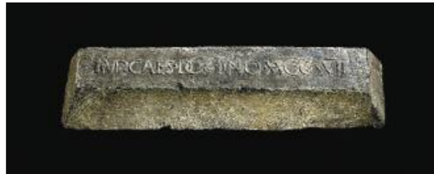
Fig 4.7 Lead pig found at Heyshaw Moor (in Nidderdale), dated to AD 81 (RIB 2404.62). The inscribed face is 508mm x 140mm. Photograph reproduced by courtesy of Bonhams, London
