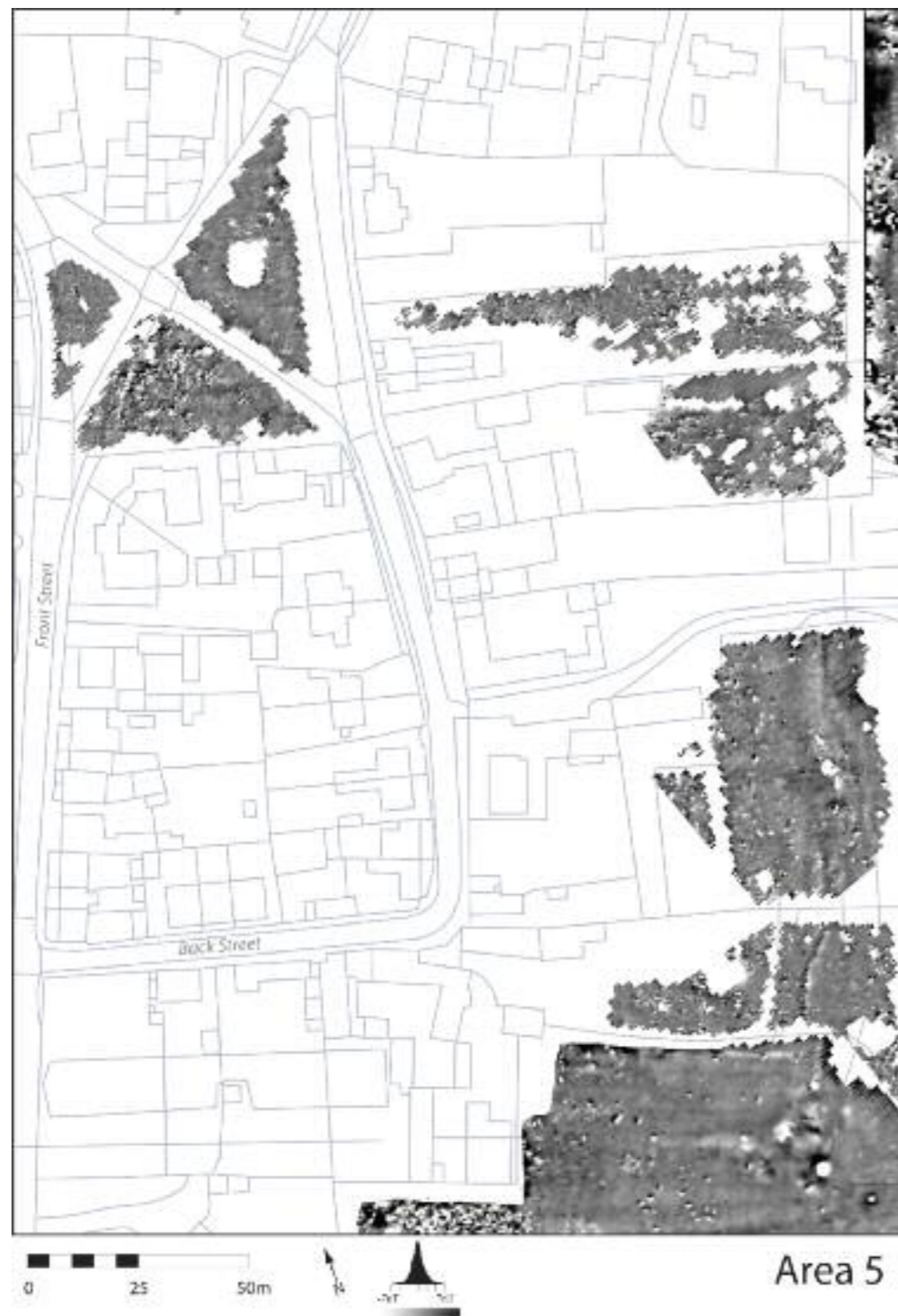
Fig 3.21 Area 5: results of the gradiometry survey in relation to modern topography. For the location, see fig 3.3. Scale 1:1500. Drawing: Rose Ferraby. © Crown copyright and database rights 2018 Ordnance Survey (100025252)
