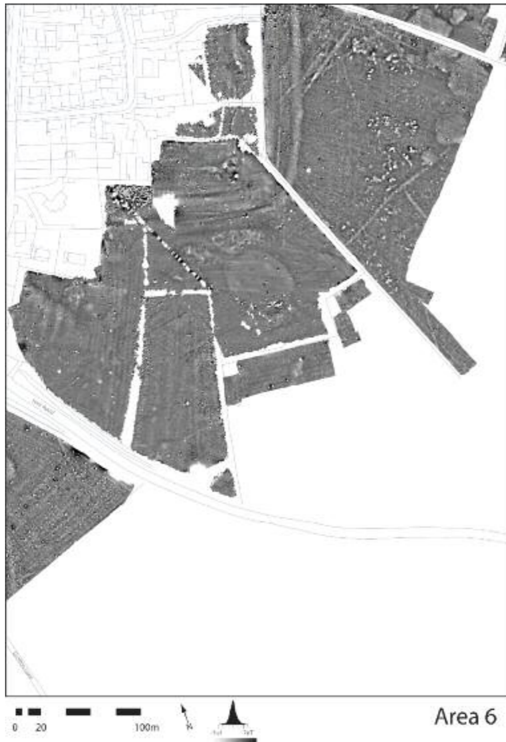
Fig 3.24 Area 6: results of the gradiometry survey in relation to modern topography. For the location, see fig 3.3. Scale 1:3000. Drawing: Rose Ferraby. © Crown copyright and database rights 2018 Ordnance Survey (100025252)
