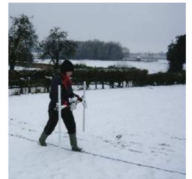
Fig 3.1 Rose Ferraby undertaking gradiometry (magnetometry) survey on site using a Bartington Instruments Grad 601 dual sensor fluxgate gradiometer. Photograph: Tom Ferraby
