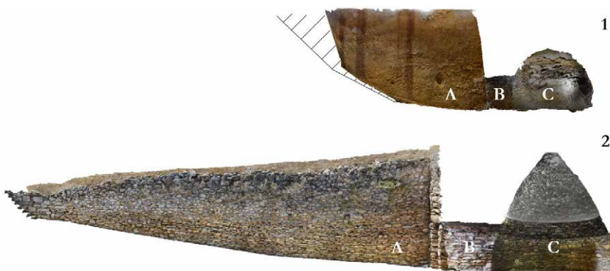
Figure 1.7. Schematic profile comparing chamber and tholos tombs, not to scale. Tripartite shape includes (a) entrance passage or dromos , (b) threshold or stomion , and (c) thalamos or burial chamber/vault. Based on textured photogrammetric models: (1) Portes chamber tomb 3 (PT3), and (2) Menidi tholos tomb (MT1).
