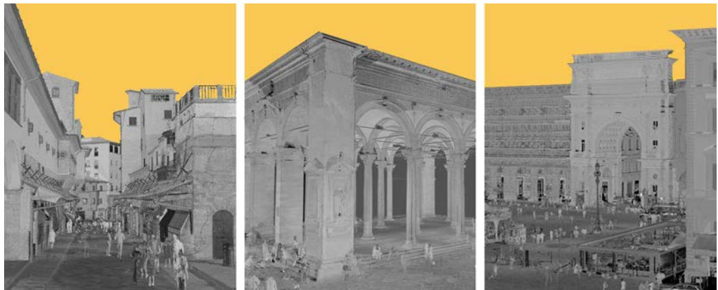
Left: point cloud of Ponte Vecchio; center: an image extracted from the points of the Piazza del Mercato Nuovo; right: an image extracted from the point cloud of Piazza della Repubblica.
