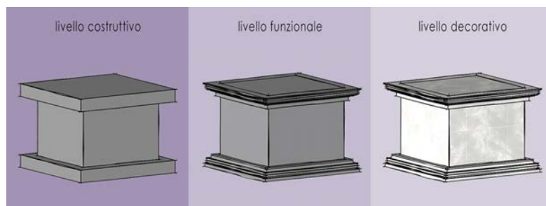
Fig. 11. Decomposition of the architectural parts of a podium according to the Vitruvian classification interpreted by Migliari.
