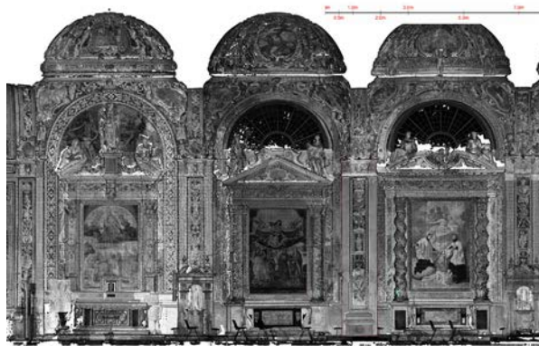
Fig. 3. Brescia, Church of Santa Maria delle Grazie, lengthwise section of left lateral nave, detail of the first and second and third chapel with photo rendering of plaster decoration of the third candelabra, signed by Giovan Antonio and Andrea Colommba, otherwise not visible due to presence of a confessional.
