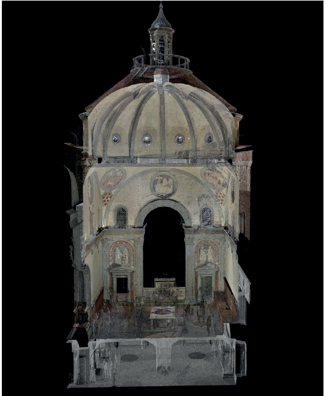
Fig.1. Sectional view of the point cloud of the Sagrestia Vecchia showing the detail of the laser scanner acquisitions.
