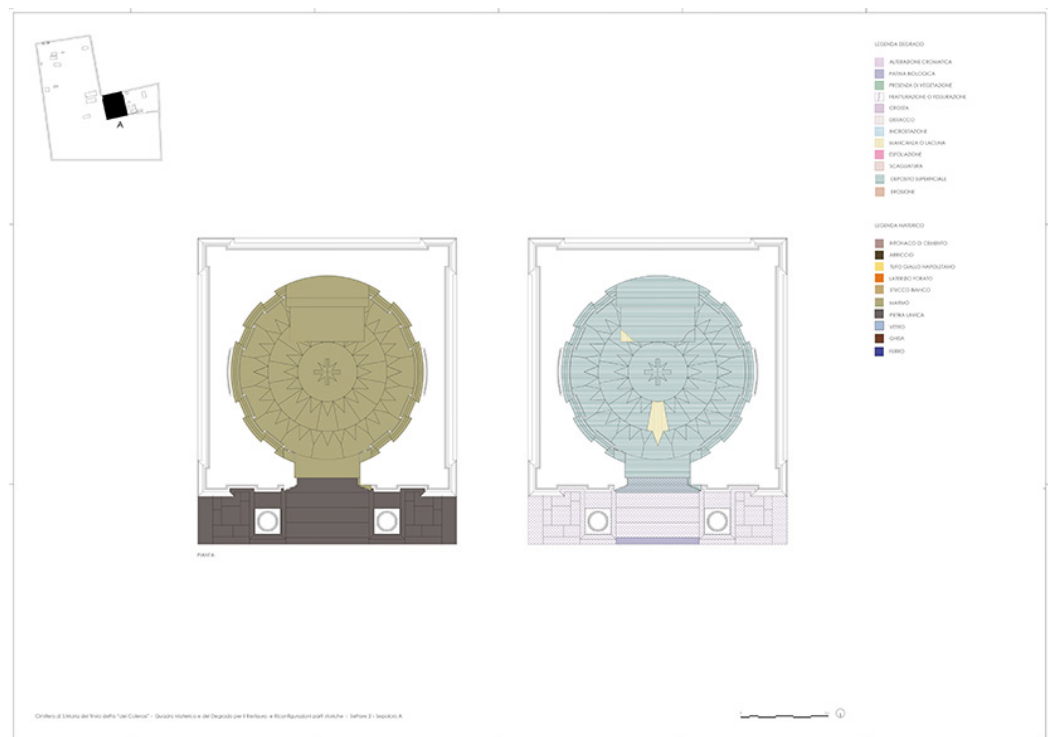
Fig. 1. The Cemetery of the Colerici in Naples. Picture of the material and degradation. Sector 2. Tomb A. Plan.
