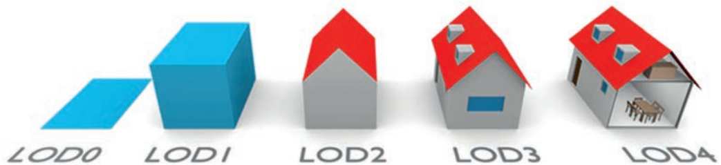
Fig. 6. Schema LODs in CityGML. [Biljecki 2016, pp. 25-37].
