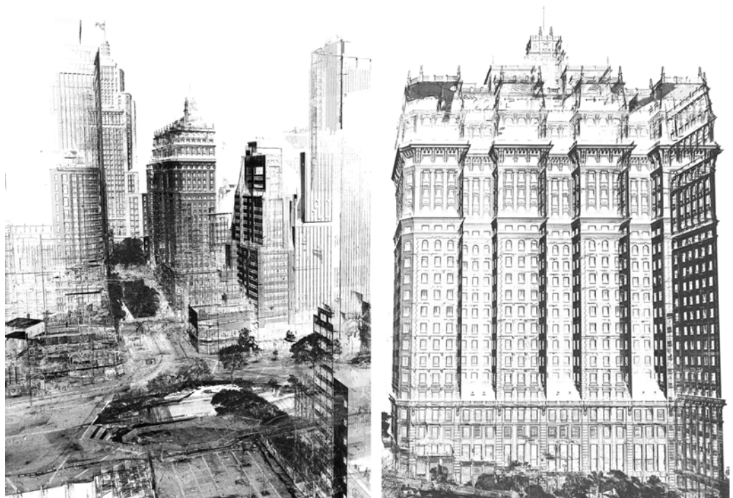
Fig. 10. Left: Point-cloud of a portion of the Avenida São João, in the historical center of São Paulo, obtained by digital laser-scanner survey in 2017. Right: detail of the point cloud with the Martinelli Building, 1934.
