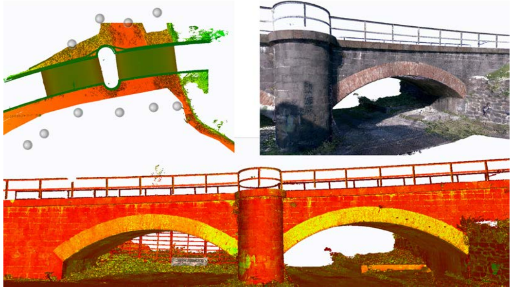
Fig. 9. On top, laser scanning survey project, right and bottom, perspective views of the point cloud.
