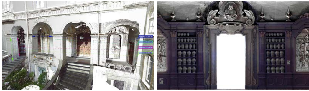
Fig. 5. Cloud cleaning and filtering, mapping with image data.
