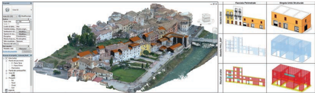
Fig. 4. From left to right: alignment of digital photogrammetric survey to BIM model and structural analysis in PROSAP [Pelliccio 2017].
