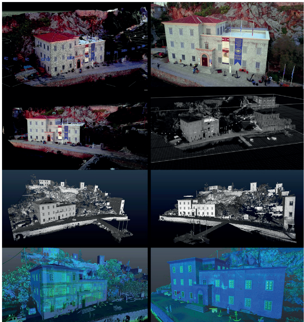
Fig. 5. The survey of the entire Museum complex was carried out using a hybrid methodology, integrating data from terrestrial laser scanners with aerial photogrammetry data to reach areas that could not be reached from the ground, such as roofs or overhangs.
