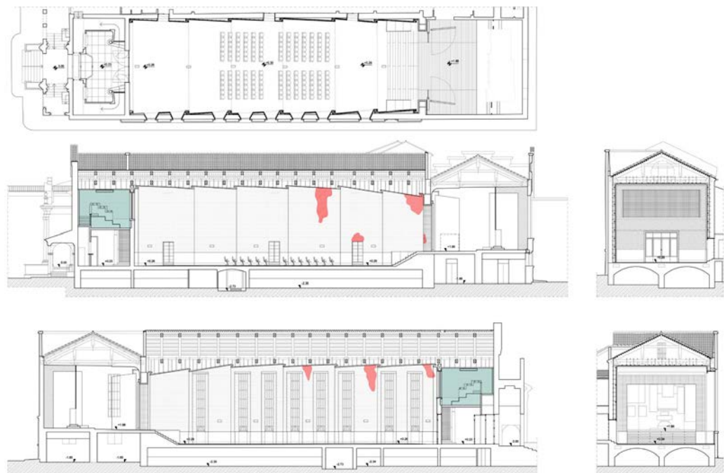
Fig. 4. The state of art of the concert hall before the restoration works. Representation from integrated digital survey, topographic survey and direct survey.
