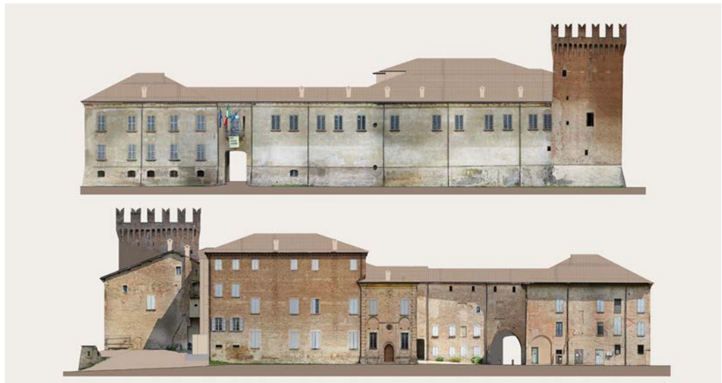
Fig. 8. North and east views of the Rocca, with ortho-photos in scale 1:50.
