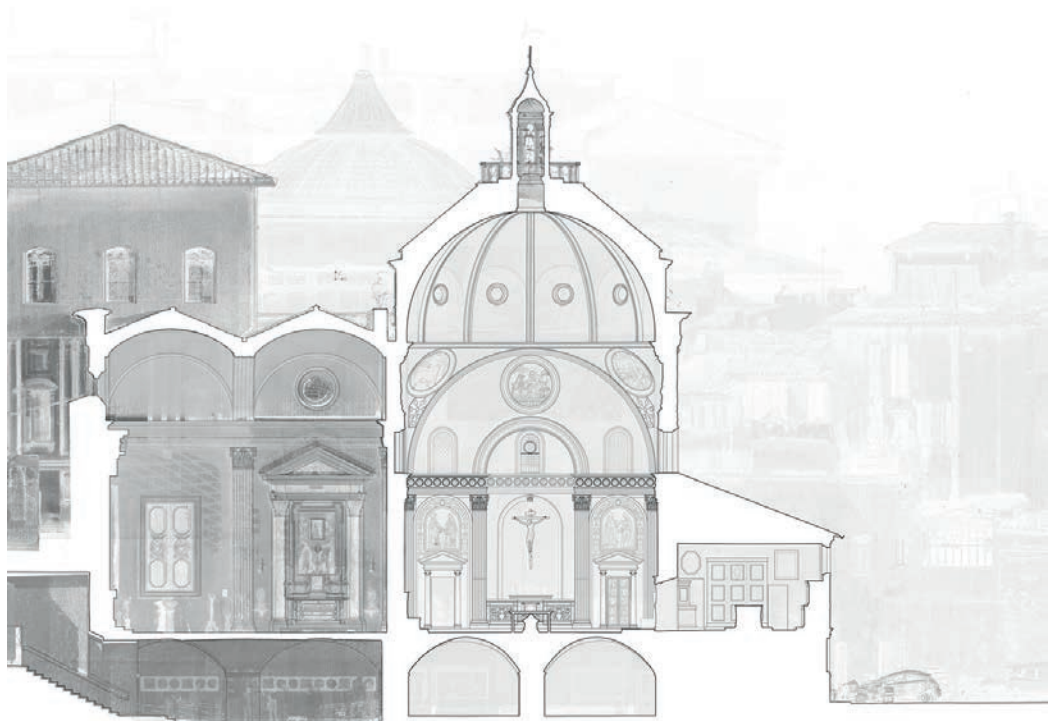
Fig. 3. Vertical section of the Sacristy showing access to the scarsella and the volumetric relationship with the surrounding structures.
