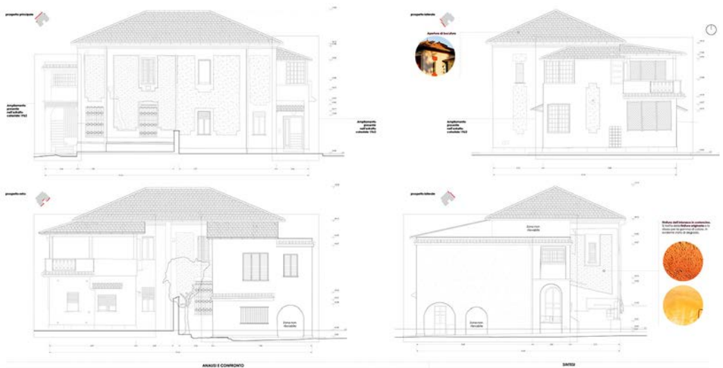
Fig. 11. Survey of the state of decay of one of the villini in the garden borough of Pigneto (graphic elaboration by V. Apostoli).
