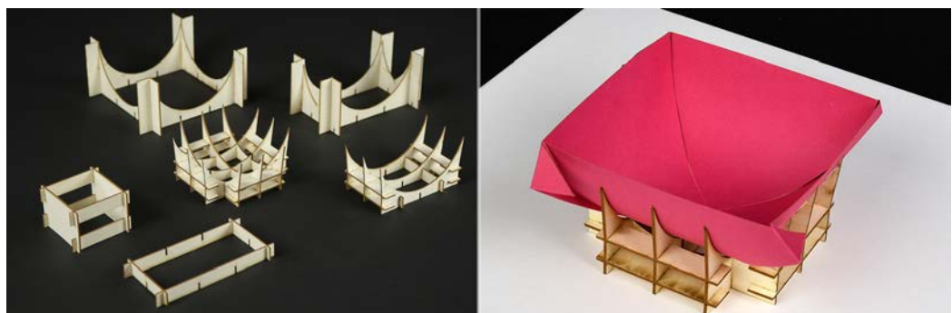
Fig. 6. Structural supports for helping the folding process and the picturing operations.
