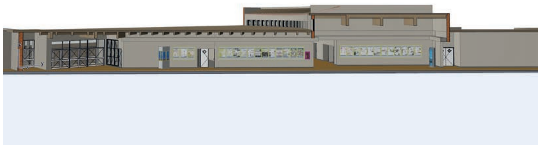
Fig. 8. Vertical perspective cross-section, model in BIM Authoring software.
