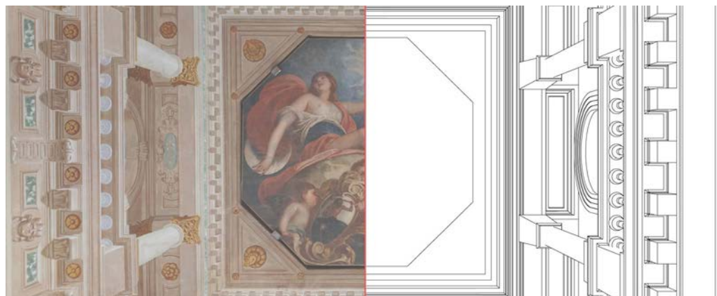
Comparison between the orthophoto of the frescoed ceiling and the virtually reconstructed pictorial space.
