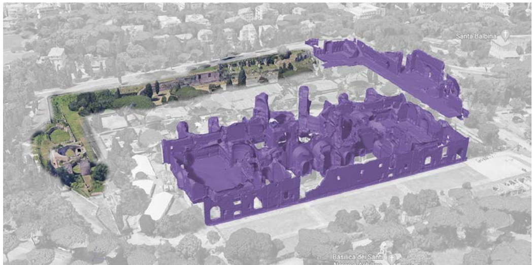
Fig. 2. In purple survey provided by the Special Superintendency for Archaeological Heritage of Rome, in color the missing area integrated with the acquisition of drone photos.
