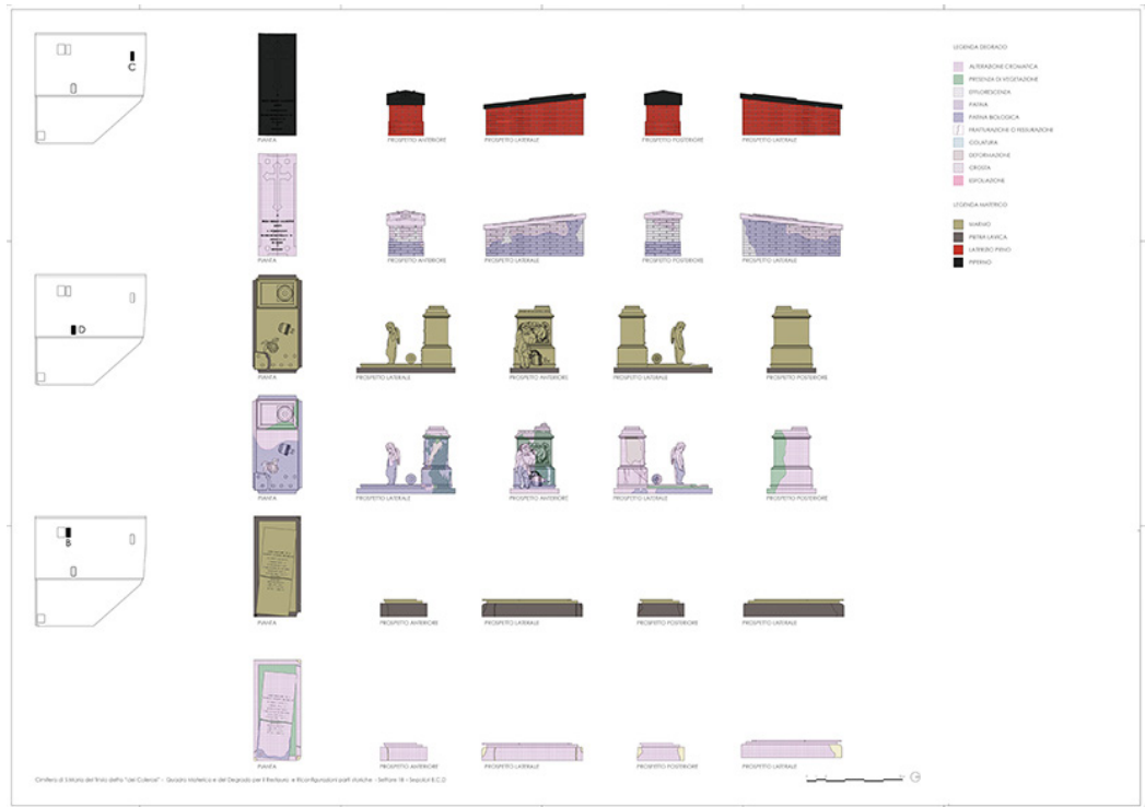
Fig. 8. The Colerici Cemetery in Naples. Material and degradation profile. Sector 18. Sepulchre B-C-D.
