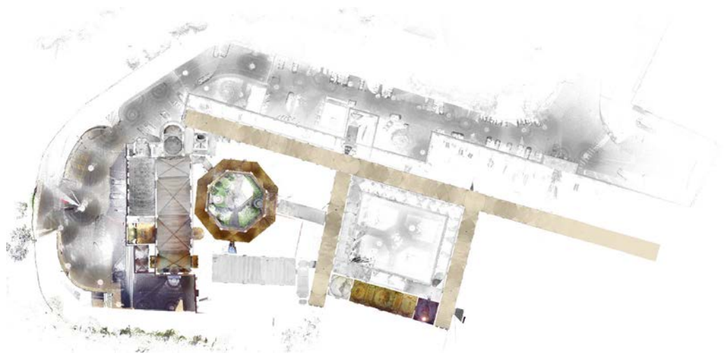
Fig. 6. Orthophoto processed by the registration of the laser scanner survey (145 scans, Scene 2020, M. Incerti). The angles were calculated with CAD software and, given the dimensions of the triangles considered (1400 by 14 meters approximately), the drawing is not graphically adequate for a canonical page of a book.
