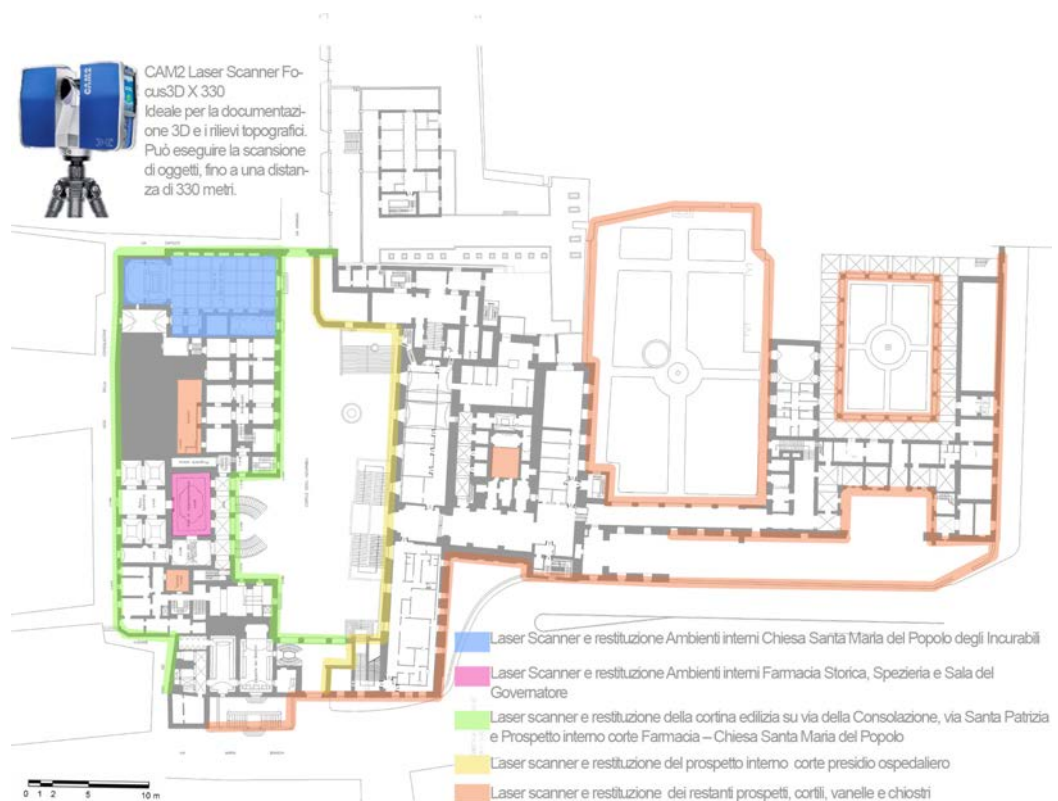
Fig. 3. The phases of investigation with laser scanner and planning for the representation of the surveyed places.
