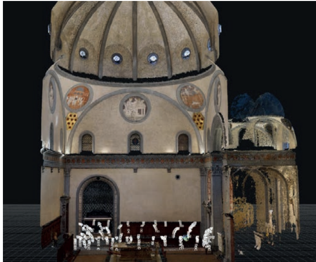
Fig. 7. Texture coming from the coloring of the models described in the previous image, the detail on Donatello's decorations made it possible to verify the correctness of the wire drawing.
