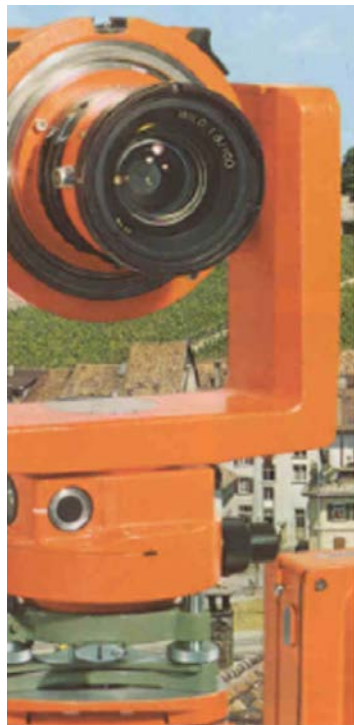
Fig. 8. On the left, Wild P31 metric camera (< http://www.wild-heerbrugg.com/photogrammetry1.htm >). On the right, calibration certificate of the camera with the scheme of the position of the fiducial points and the main points of symmetry and self-collimation with respect to the central cross impressed on the film.
