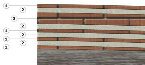
1. LB-Rasilla: Rasilla in laterizio 15x30x1.5 cm 2. LB-Concrete: Malta cementizia / calce sp. 2-3 cm 3. LB-Tabique: Tabique in laterizio 15x30x4.5 cm
