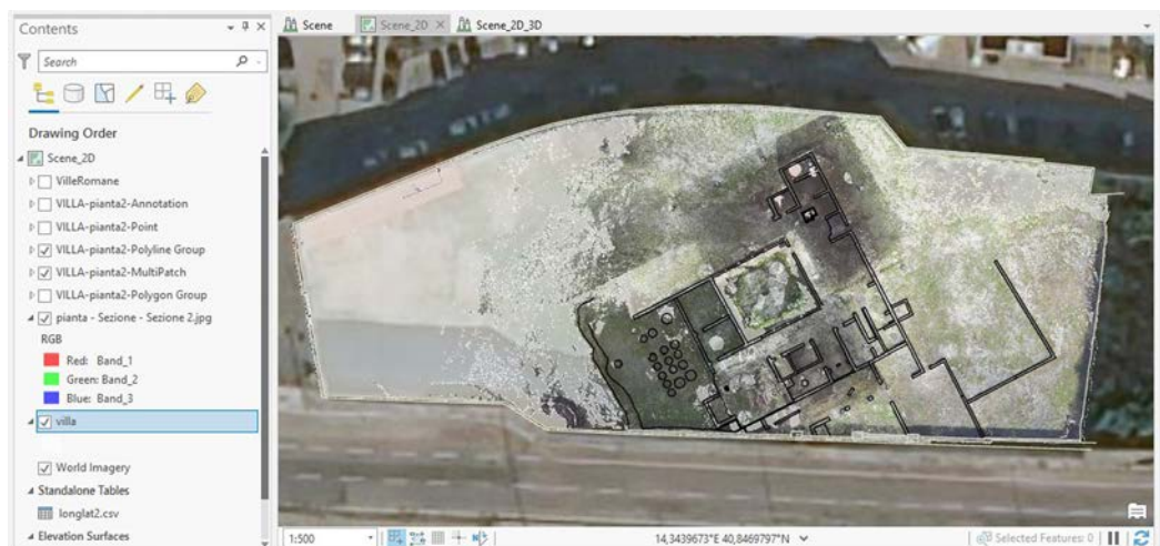
Fig. 10. Orthophoto and plan of the Roman villa of Ponticelli in GIS environment.
