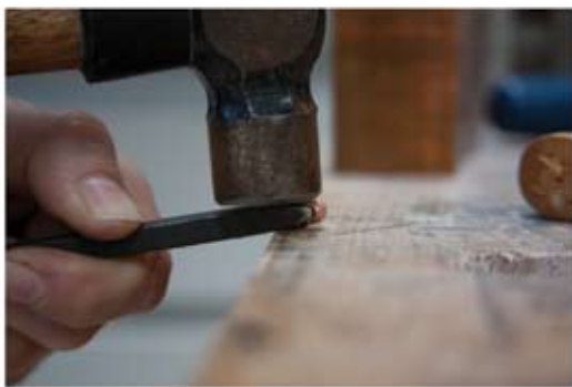
4 Straighten the legs and yield the final shape by hammering the stud around the punch.
