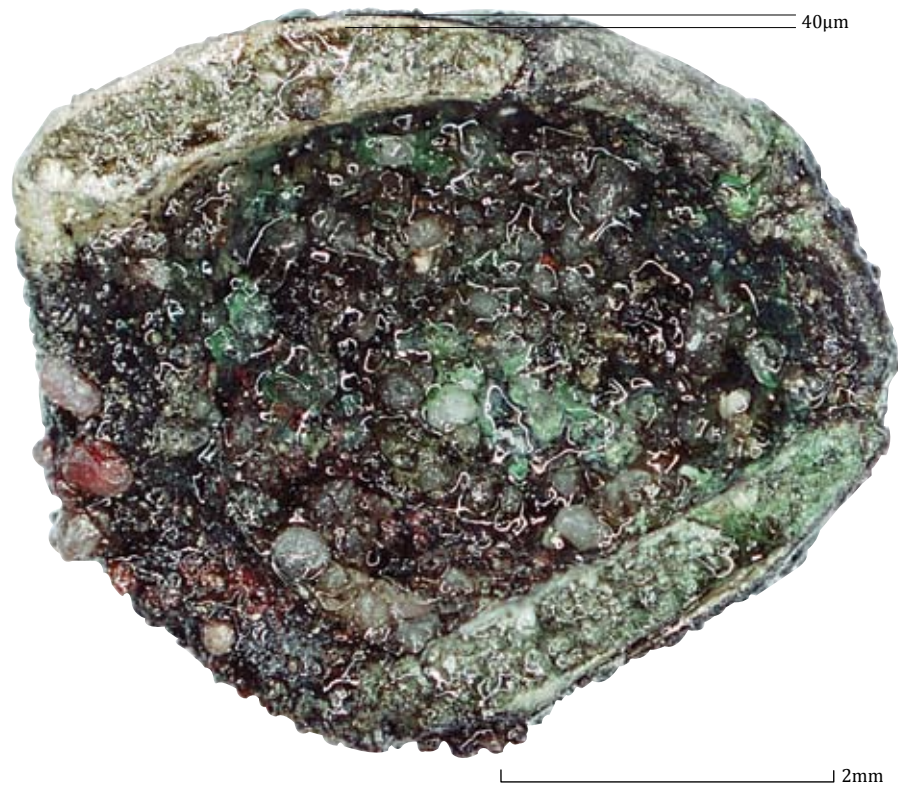
Fig. 9.3 A look at the inside of the head of a stud. Due to fracture of the legs, the cross-section shows a white outer layer of about 40 \mu\text{m} thick. Also, grain-like green and red products can be seen. Figure by J. Nienhuis/J. van Donkersgoed.
