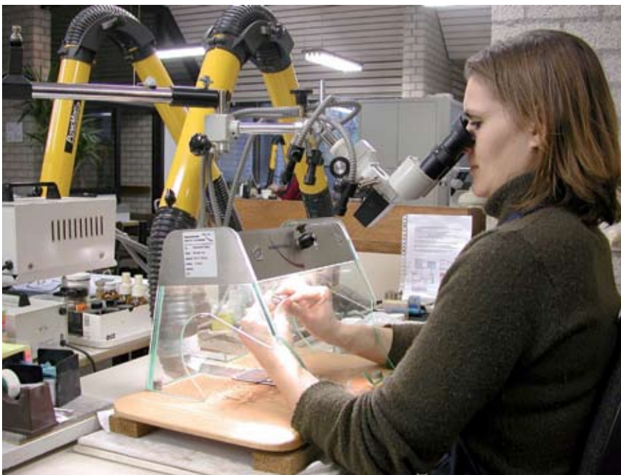
Fig. 8.14 The manual cleaning of the finds under the binocular microscope. Figure by Restauratieatelier Restaura, Haelen.
