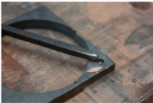
3 Place the punch on the template, above a preformed hole, and hit it.
