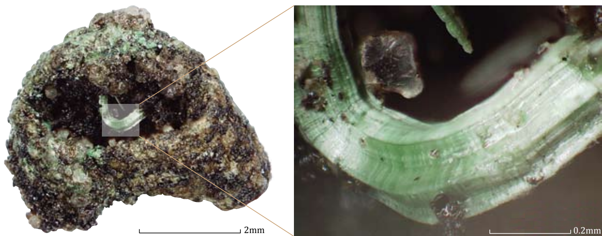
Fig. 9.4 Small stud showing the unique curly shape of malachite, a pale green copper corrosion product. Figure by J. Nienhuis/J. van Donkersgoed.
