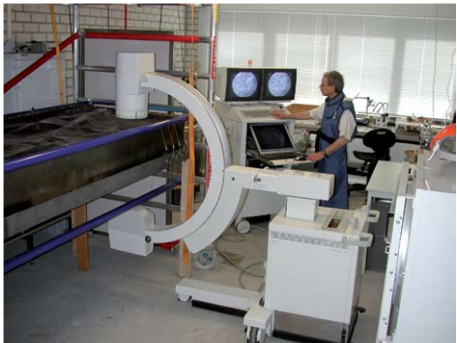
Fig. 8.9 V 1003 suspended in a frame whereby the X-rays are taken using a C-arch. Figure by Restauratieatelier Restaura, Haelen.
