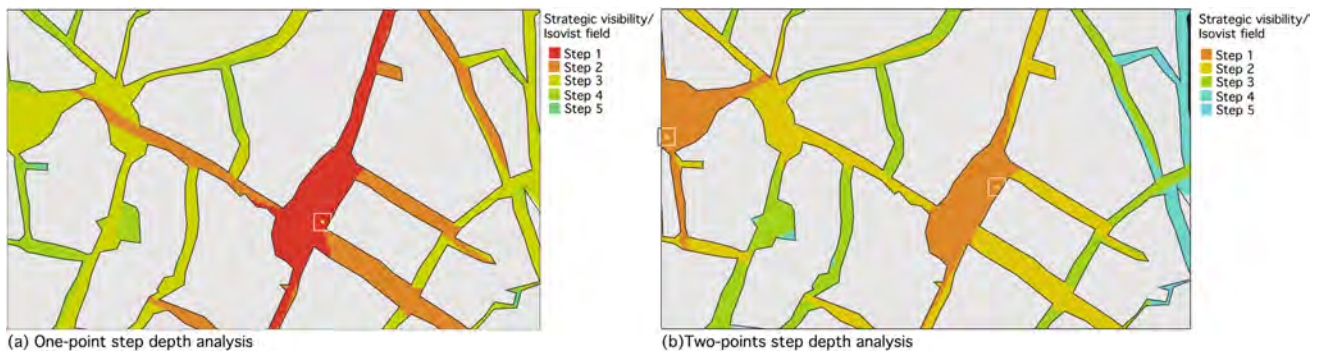
Fig. 3.16 Point-step depth analysis from one point (a) and two points (b) from an ancient area from 1300 in the centre of Sofia, Bulgaria
