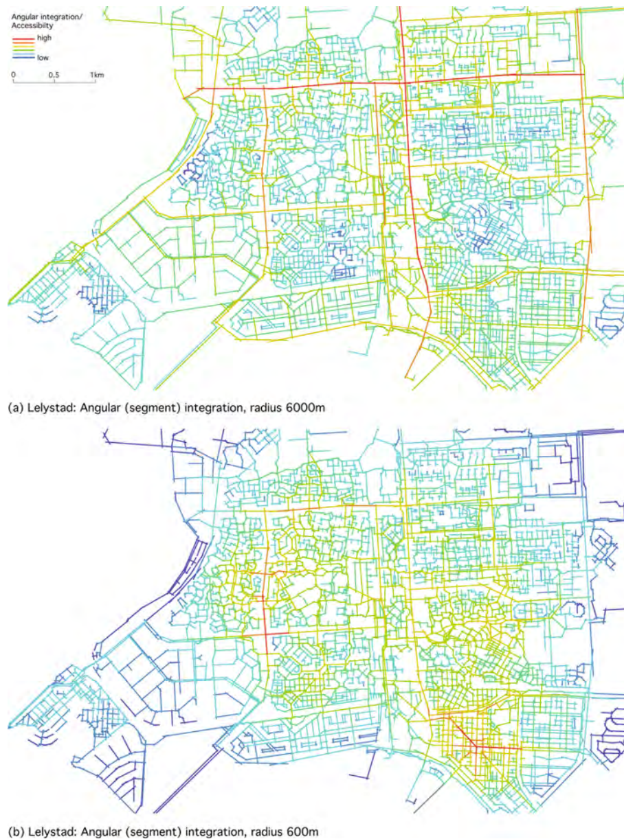
Fig. 2.41 Angular (segment) integration analysis for the town of Lelystad with (a) a radius of 6,000 m and (b) a radius of 600 metres
