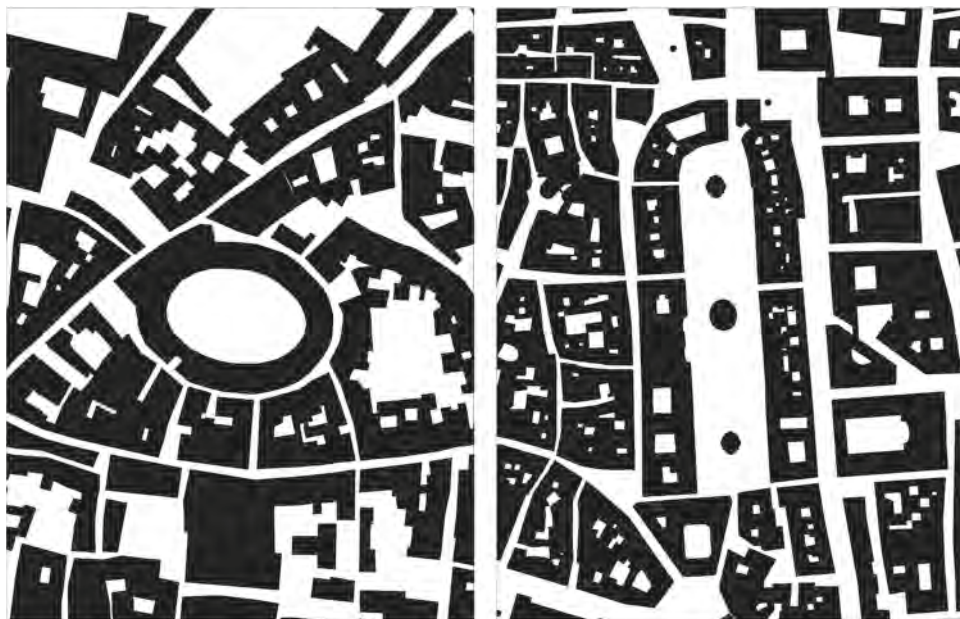
Fig. 1.16 An amphitheatre’s influence on the urban pattern in the Italian town of Lucca (left), and an ancient Roman stadium’s influence on Piazza Navona’s built form in Rome (right)
