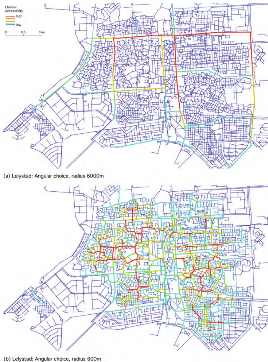
Fig. 2.37 Angular choice analysis for the town of Lelystad with (a) a radius of 6,000 m and (b) a radius of 600 m
