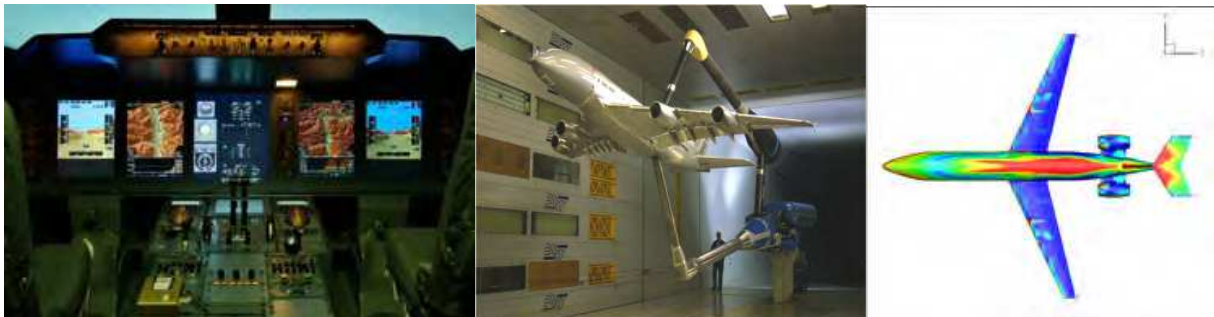
Fig. 14. Left: Future integrated “intelligent” flight deck for safe and efficient operation in nominal and adverse conditions. Mid and right: application of wind tunnels and CFD to acquire accurate aerodynamic estimates for simulation of flight outside the normal envelope, aircraft damage and icing to mitigate in-flight loss-of-control
