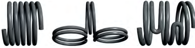
Figure 5.17: Coiled configurations: horizontal coil (left), Coiled Flow Inverter (center), Coiled Flow Reverser (right, European patent No. 19176360.6-1019, EP3741453 A1).
