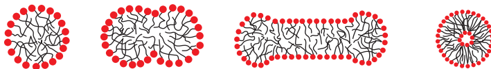
Figure 3.33: Schematic representation of surfactant aggregates (spherical, globular or rod like micelles, or spherical bilayer vesicles) in dilute aqueous solutions [170].
