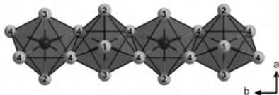
Figure 2 Strands of edge-connected [\text{TmF}_7]^{4-} polyhedra according to 1\text{D}-[\text{Tm}(\text{F}_{1,2,3})_{3/1}^t(\text{F}_4)_{4/2}^e]^{2-} propagating along the b -axis in the crystal structure of \text{K}_2\text{TmF}_5 .
