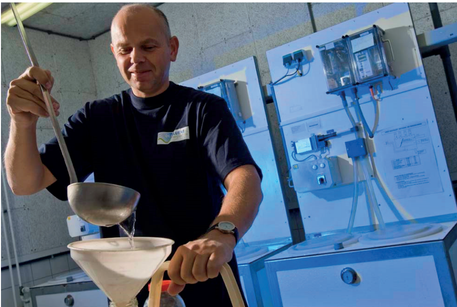
Figure 15.27 Effluent sampling at WWTP Houtrust (Photo: Delfluent Services BV).
