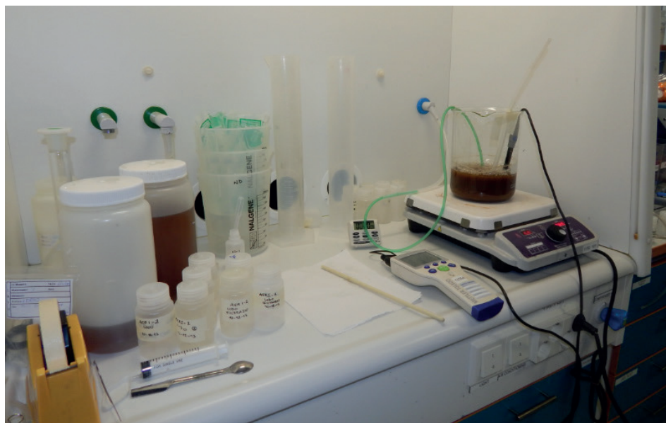
Figure 16.7 Aerobic batch set up assembled at the pulp mill laboratory facilities (Photo Bentancur S.).
