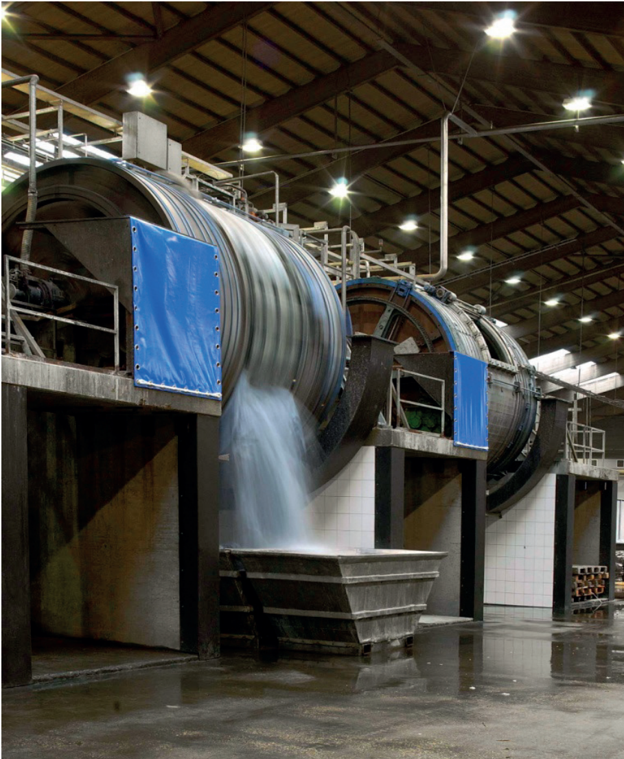
Figure 9.4 Part of the leather treatment process at Ecco Tannery Holland BV (Photo: Moussa M.S.).
