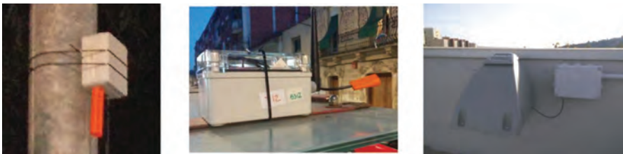
Figure 7.10 Sensor devices. Barometric wake-up device ( left ). Temperature, humidity and light wake-up device ( center ). Airbase WLAN air quality device ( right ).
