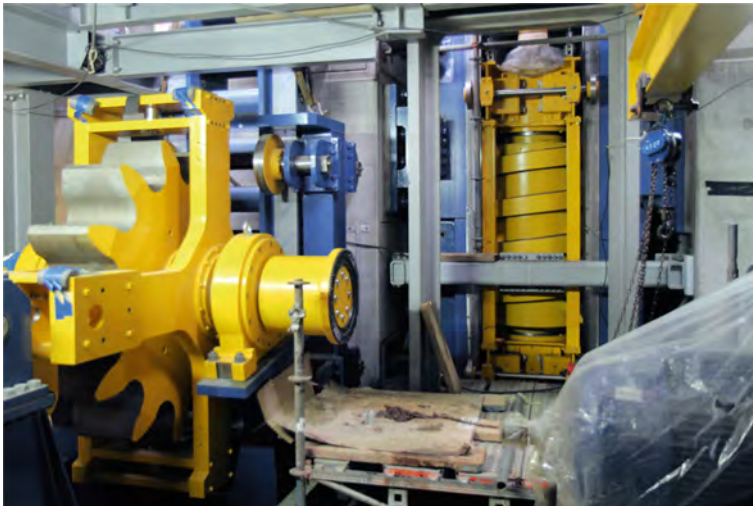
Fig. 18. Photo of gear rack and nut post
