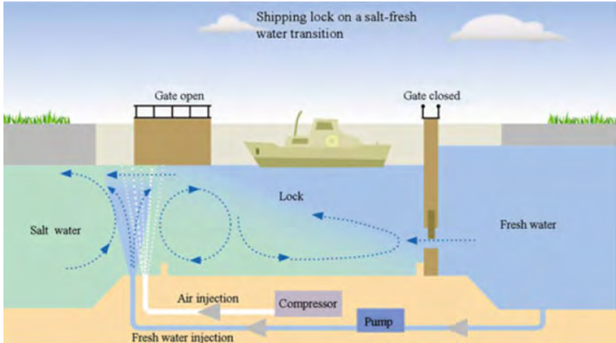
Fig. 3. Schematic representation of the options which have been investigated for the Krammer locks, including bubble screen, water screen, flushing discharge and raised lock sill. (From Keetels et al. 2011)
