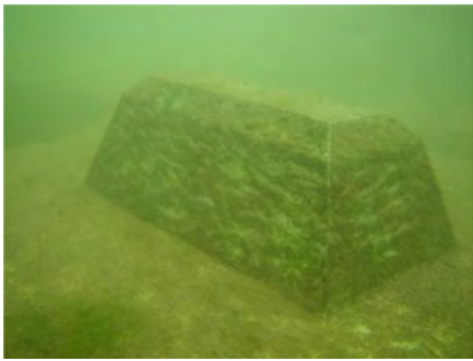
Photo 7. Attached algae on EAC panel
