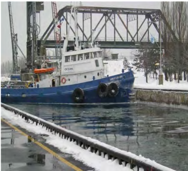
Fig. 2. Ice removal with a customized ice scraper tug
