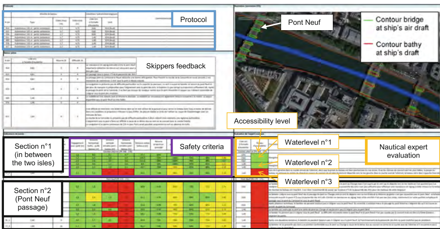
Fig. 6. Extract from a simulations sheet for a 135 m × 11.4 m container ship sailing downstream with a draft of 1.7 m. Analysis of the section n°1 and n°2 of the waterway.
