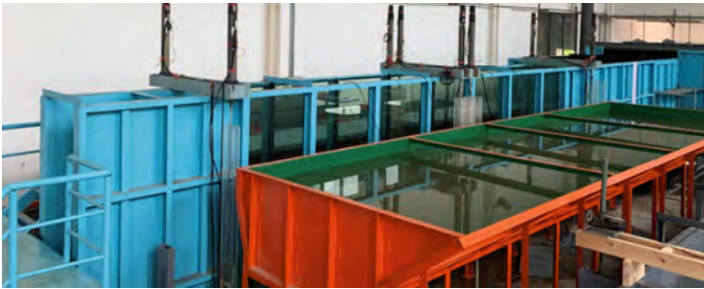
Fig. 4. The overall physical model of filling and emptying system of ship lock with trapezoidal section pools
