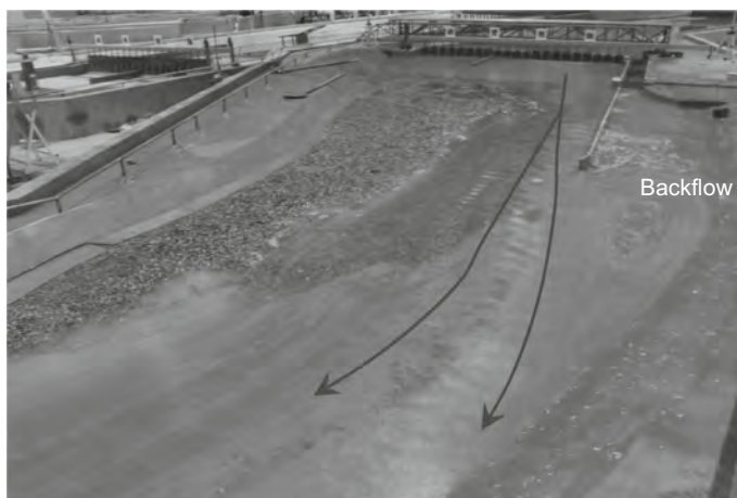
Fig. 4. Downstream flow regimes of initial layout ( Q = 1000 \text{ m}^3/\text{s} )
