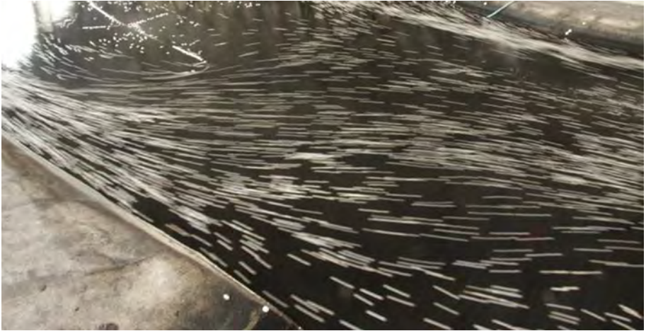
Fig. 5. Local flow pattern at the head of Daijiazhou sandbar under low flow ( Q = 7310 \text{ m}^3/\text{s} )
