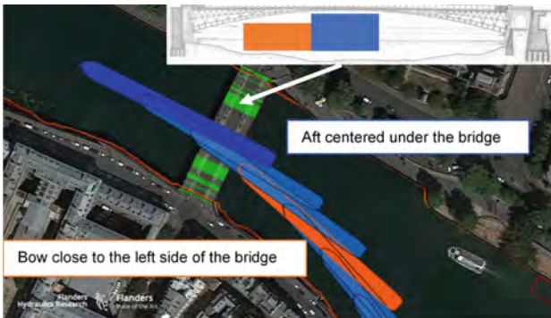
Fig. 8. 125 m ship passing the Pont d'Arcole in Paris.
