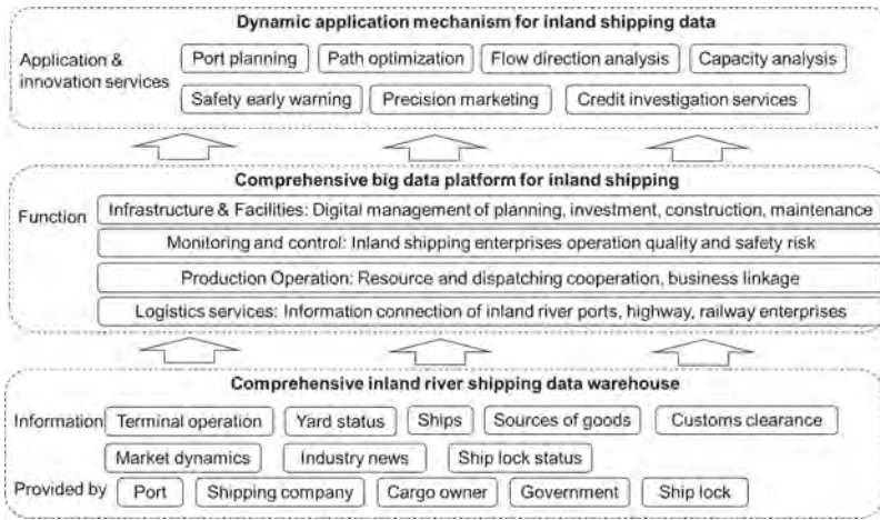
Fig. 1. The structure of comprehensive big data platform for Zhejiang inland shipping based on integrating “four-port linkage” information.
