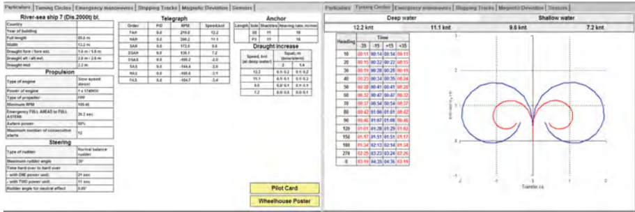
Fig. 1. Basic data of River-Sea ship, simulator Wärtsilä NT PRO 5000
