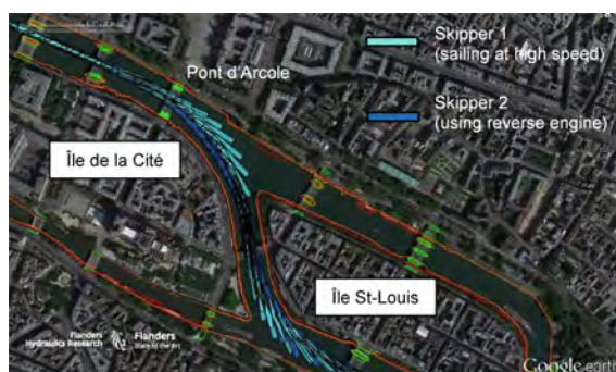
Fig. 10. Simulations with a 125 m long ship sailing in current.
