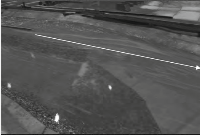
Fig. 6. Flow regimes of downstream entrance area with dredging flood plain to 65 m elevation ( Q = 1000 \text{ m}^3/\text{s} )
