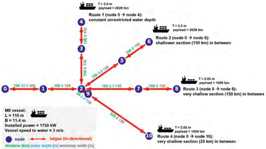
Fig. 3. OpenTNSim input: vessel properties and graph information.
