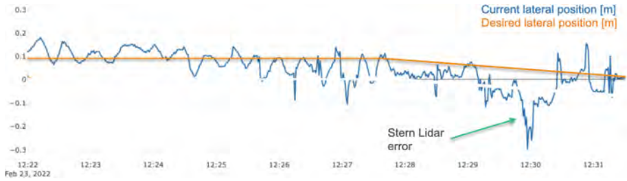
Fig. 3. Desired and estimated lateral positions
