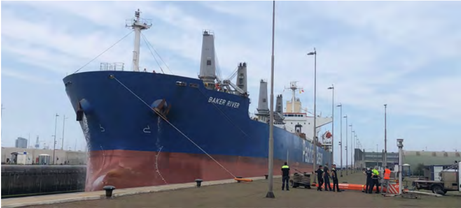
Fig. 3. Setup of the ShoreTension system (orange cylinder). Note that the number of people in the picture is not representative for the personnel needed to operate the system, as this picture was taken during one of the first “instruction” measurements.
