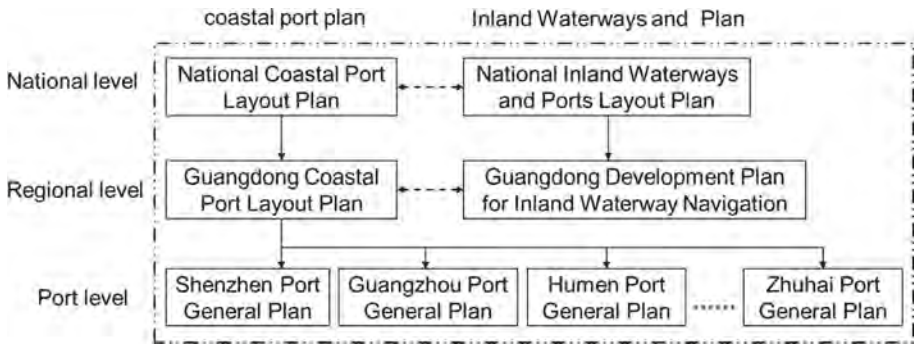
Fig. 5. Diagram of the port and waterway planning system.
