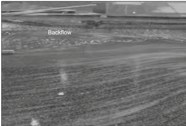
Fig. 5. Flow regimes of downstream entrance area with dredging flood plain to 67 m elevation ( Q = 800 \text{ m}^3/\text{s} )
