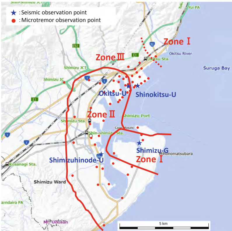
Fig. 4. Zones with similar seismic characteristics (Example: Shimizu Port)
