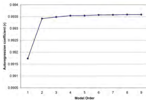
Fig. 4. The correlation coefficient for different orders regarding the AR model which was used for water level simulation
