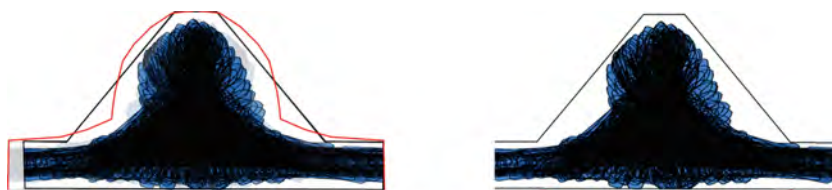
Fig. 11. Principle of the optimization of the small trapezoid (in red), optimized geometry on one bank only (left): rounded top and opening from the channel following the approach paths and optimized geometry using both banks (right): widening of the channel on the opposite bank
