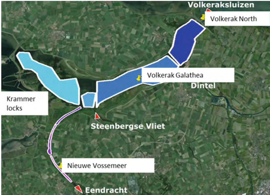
Fig. 5. The schematization of lake Volkerak-Zoom in the WANDA-Locks model. The Krammer locks are modelled in detail and provide fluxes and concentrations into the box at the west (left) side.
