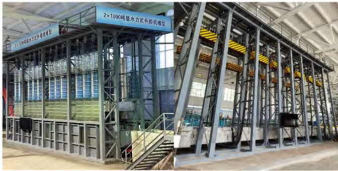
c) Hydro-floating ship lift (2×1000t)
