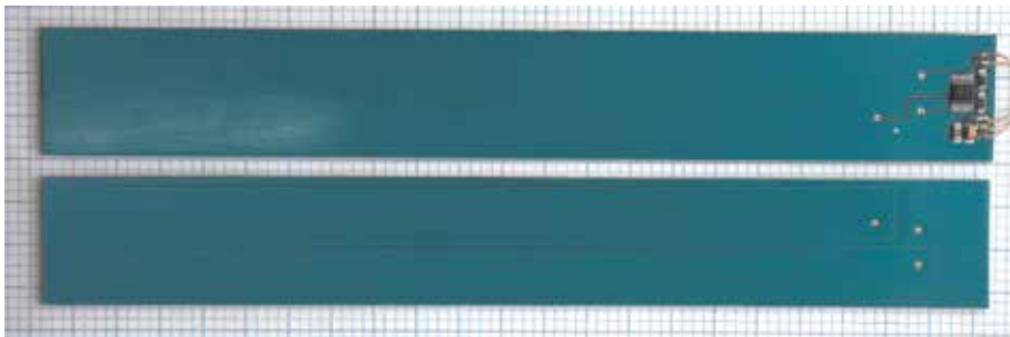
Figure 8. Realized sensors in the department of electric and magnetic measurements of IED NASU: top – reverse side of the sensor; bottom – operational side of the sensor with working electrodes.
