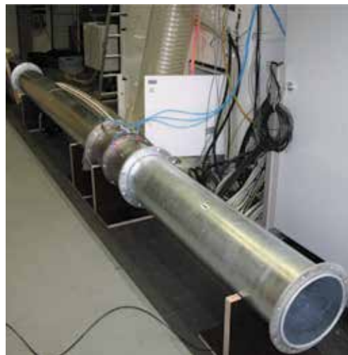
Figure 6. Volumetric flowrate calibration measurement section.
