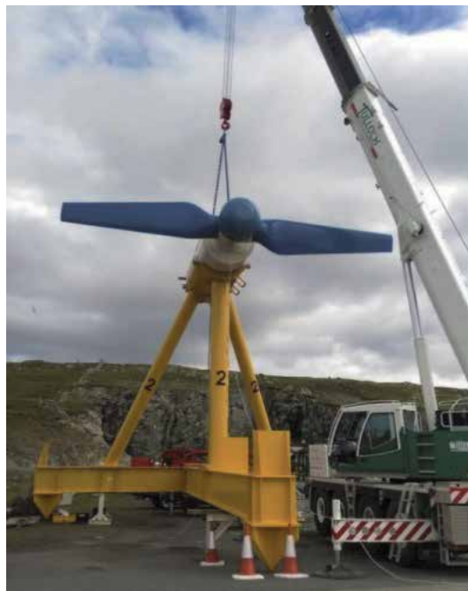
Figure 2. Nova M100 tidal turbine (Source: ©Nova Innovation).
